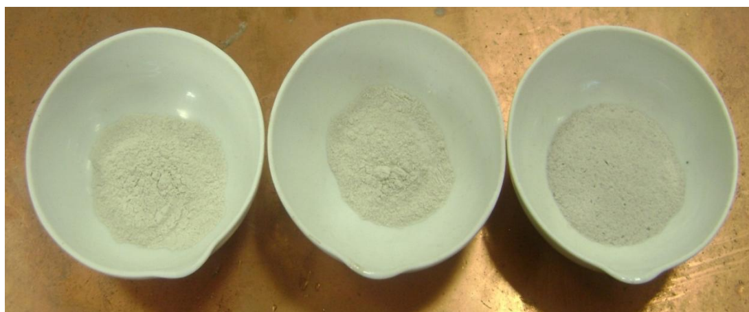
Figure 3.4 Bentonite modified by AA at 30°C for 3h with acid concentration of 0.075M, 0.1M and 0.5M.
