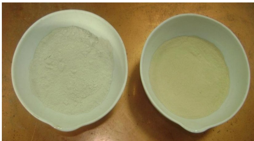
Figure 3.3 Bentonite modified by TA at 100°C and 500°C for 20 min
