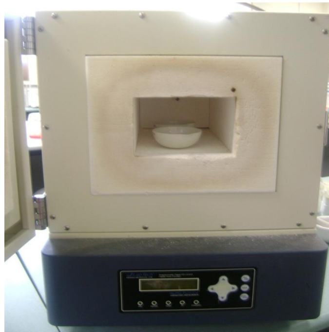
Figure 3.2 Muffle furnace used for thermal activation of bentonite
