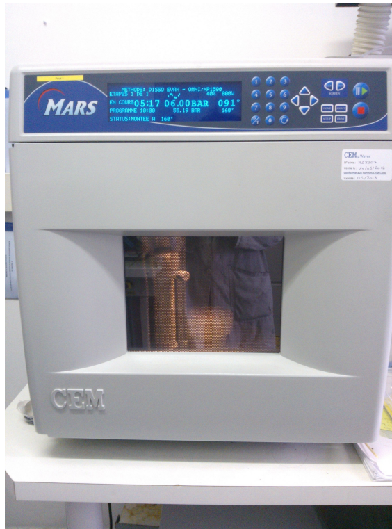
Figure 4.6: CEM MARS5 microwave
