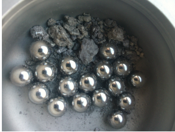
Figure 4.3: TiH 2 sponge with stainless steel balls in a ball mill vial
