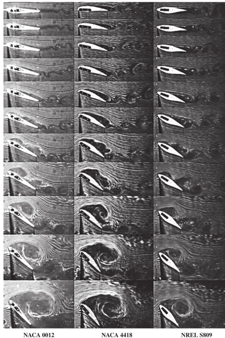
Fig. 14. Flow structures around the NACA 0012, NACA 4418 and NREL S809 airfoil undergoing constant pitch dynamic stall to a maximum angle of attack of 50° at a Reynolds number of 10,000 and a reduced frequency of 0.1. Each subsequent sequence represents an increment of 5° starting from an angle of attack of zero degrees.
