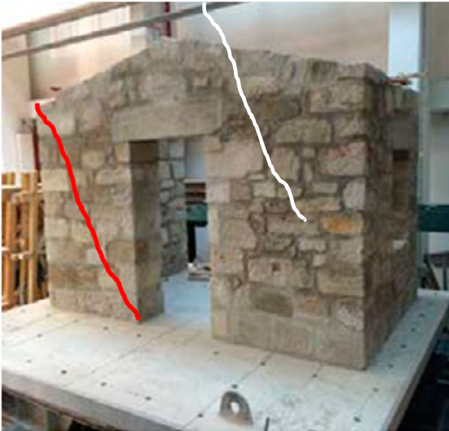
Figure 2: Failure mechanism of the stone building
