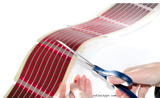
Figure 1.2: A commercially available organic solar cell † manufactured through a roll-to-roll printing method.
