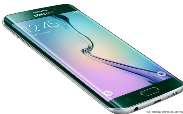
Figure 1.1: An OLED display on a mobile phone.* Reduced power consumption and increased contrast are two significant advantages over liquid crystal displays (LCDs) in this application. The curved edges on this model demonstrate the flexible nature of the display panel.
