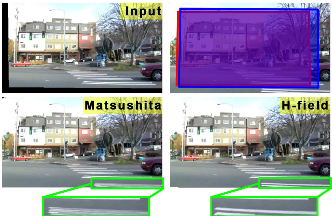
FIGURE 5.13: Selected video inpainting result 2. (top left) Updated input frame \tilde{I}_t ; (top right) Blue and red shaded windows respectively indicate equivalent final output frames of Grundmann et al. [55] and Liu et al. [89] who do not conduct video inpainting; (bottom left) Matsushita et al. [98]’s result using motion inpainting; (bottom right) Result using homography fields.
