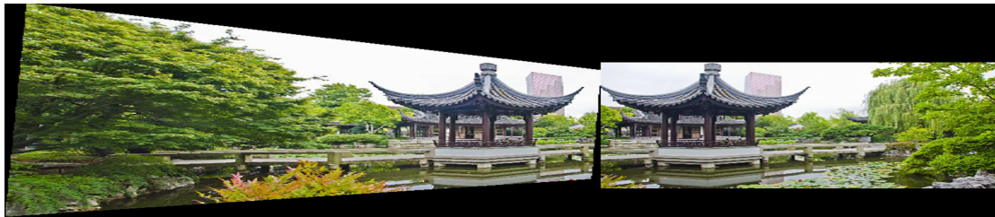
(a) Pre-warp input images using a homography estimated from SIFT keypoint matches.
