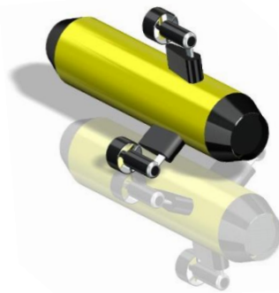
Figure 1.6: Rendered CAD model of the prototype AUV. The vehicle is equipped with three bi-directional thrusters, which sit on three wing-profiled bases attached to the hull.
