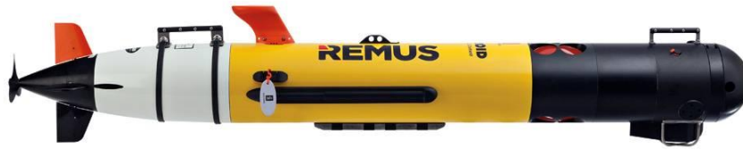
Figure 1.4: REMUS 100 AUV (WHOI, 2009). The vehicle is equipped with a rudder and stern planes for maneuvering, a vertical thruster for depth control and a propeller for speed control.
