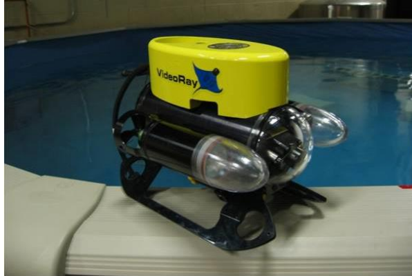
Figure 2.3: Micro ROV - VideoRay Pro III (Wang, 2007). The micro tethered ROV has two horizontal thrusters and a vertical thruster.
