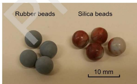
Fig. 2. Rubber and silica beads used in the damping ratio calibration.
