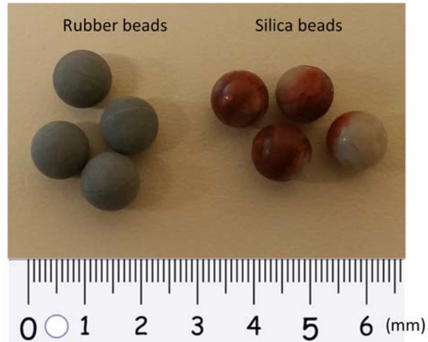
Figure 4-2. Rubber and silica beads used in the damping ratio calibration.
