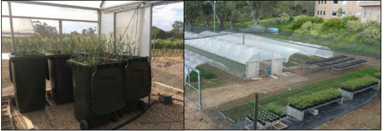
Supplementary Figure 5. Set up of the deep soil platform. On the left, 1 m deep wheelie bins were used to mimic a deep soil profile as in natural conditions in Northern Mexico. On the right, wheelie bins were located under a polytunnel to avoid any rainfall and increase temperature. Plants were irrigated until booting to let the bins dry up. Soil moisture was recorded with gypsum blocks located at 10 and 40 cm depth. Temperature and humidity were recorded using dataloggers.
