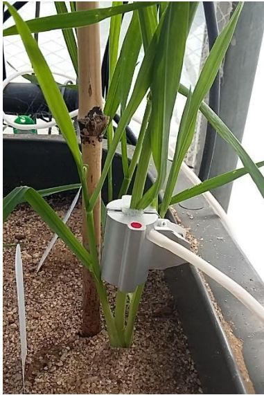
Supplementary Figure 3. Sap flow sensors, located on the main tiller, were used to measure heat pulse velocity every 15 minutes at the stem level during both days and nights.
