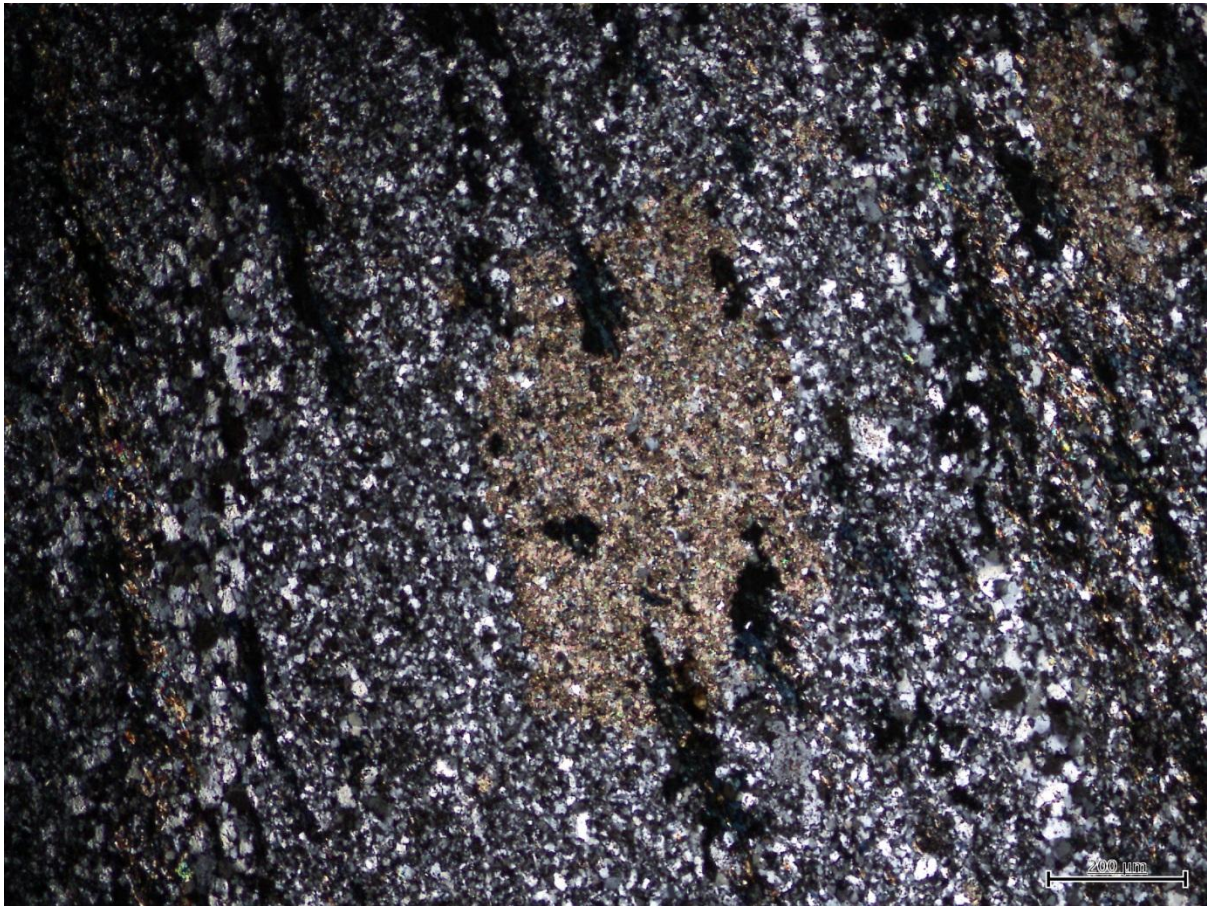
Figure 57: Over printed calcite in a fine grained matrix of quartz with foliated chlorite
