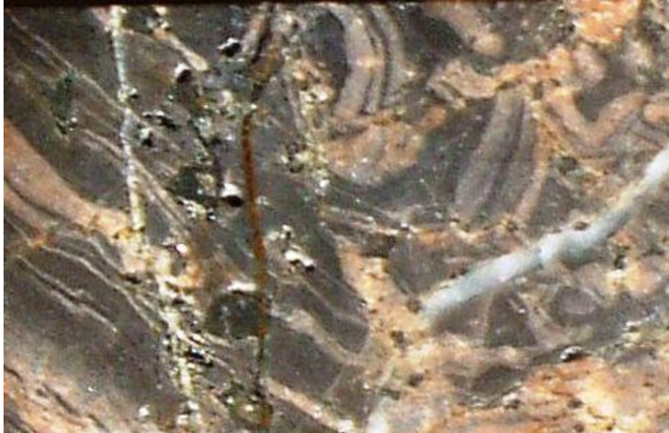
Figure 12: MC002DD 3-29.00m. Fine grained folded bedded volcanics/metasediments??, brecciated and network veined by quartz-albite veining . Minor albitisation of host rocks (pinking) and late quartz (grey). Slab. WOF 3.6cm.
