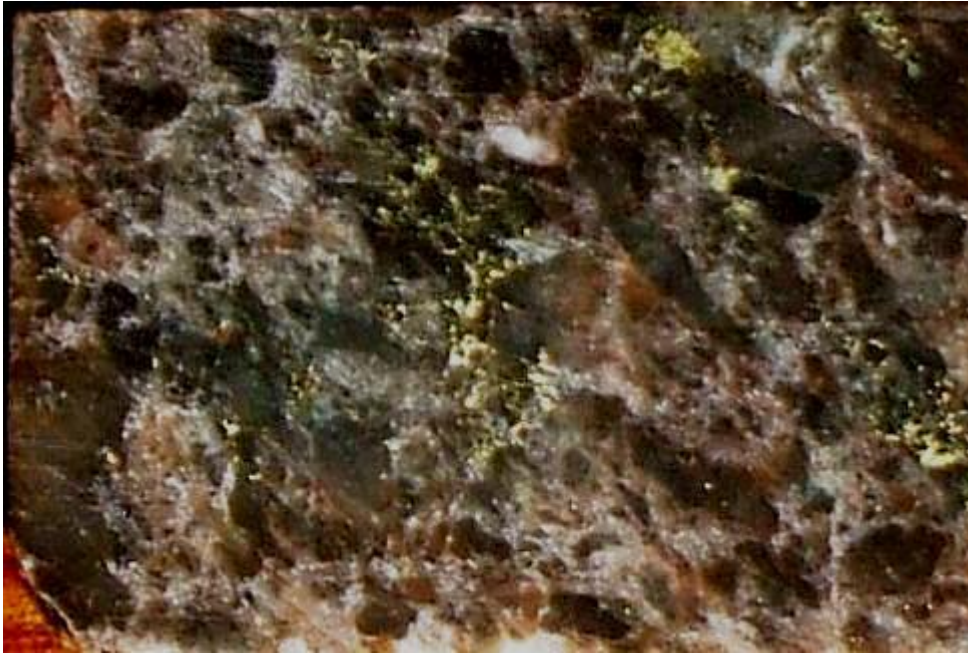
Figure 8: MC001DD 37-422.00m. Early albite (pale pink) in fine grained host rock brecciated and overprinted by carbonate network veining (white) and late wispy chalcopyrite (yellow). Slab. WOF 3.6m.
