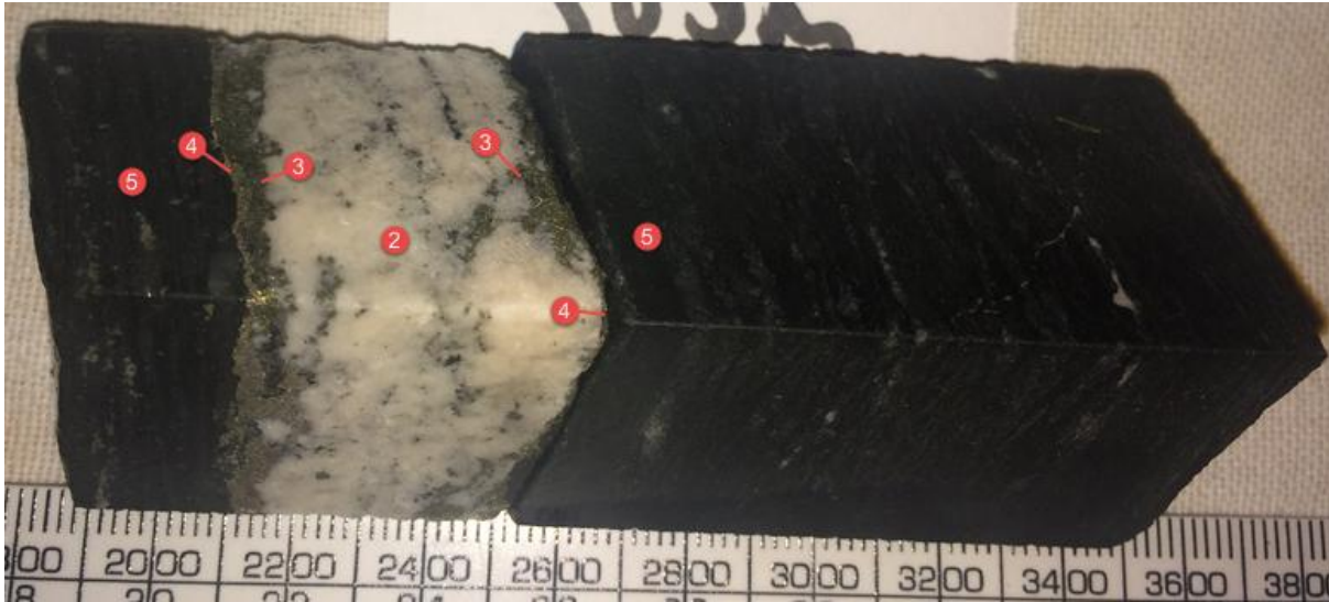
Figure 55: Mineralisation (py=cpy) at edge of calcite, in boundin neck? (1). Order: calcite(2)>cpy(3)>py(4)>chl (5)
