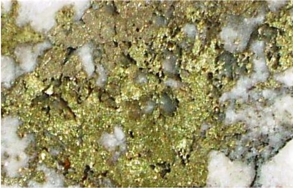
Figure 16: MC003DD 12-83.80m. Dolomite, broken and overprinted by chalcopyrite-pyrite (yellow). Pyrite-slightly less yellow , ( top left). Slab 3.60cm.
