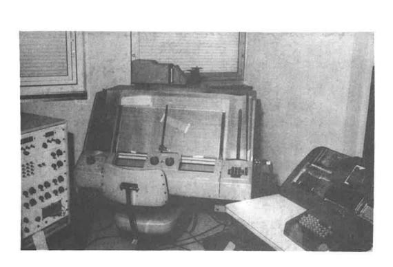
Figure 7 Recording equipment Left - the digital converter unit, Centre - the record reader showing projector viewing screen and reading head, Right - the IBM 26 punch card unit.
