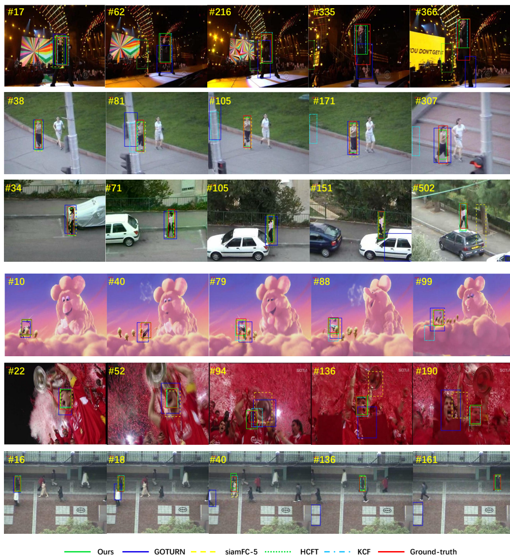
FIGURE 4.9: Tracking results comparison on some key frames of 9 representative OTB-100 video sequences. The comparing methods include the proposed CODA tracker (green), GOTURN [5] (blue), Siamese tracker [6] (dashed yellow), HCF tracker [7] (dashed green) and the KCF algorithm [8] (dashed light blue). The red bounding boxes are the ground-truth locations of the tracking targets. Better view in color.
