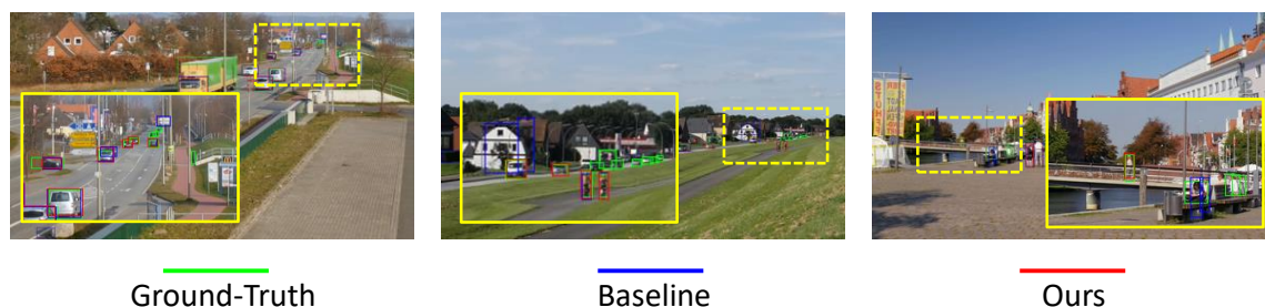
FIGURE 3.9: Qualitative results on the proposed SHV dataset (best viewed in color), visualisation threshold was set to 0.75. Bounding boxes showed in green, blue and red represent ground-truth annotation, detection results of baseline Faster R-CNN-R50 and the proposed Faster R-CNN-R-50-ours respectively.
