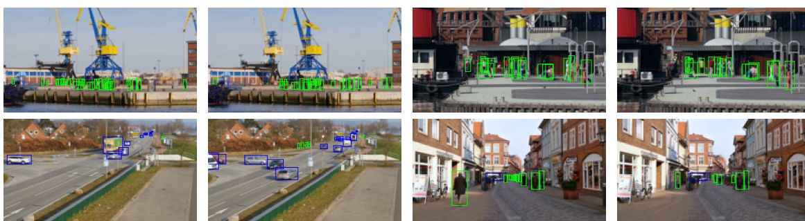
FIGURE 3.8: Preview of the SHV dataset, the green and blue bounding boxes represent the annotated objects of “human” and “vehicle” super category respectively (ignore regions are not shown here). It should be note that, the images included in the dataset have a 960 \times 540 resolution, here we have resized the images to a very low resolution for preview.
