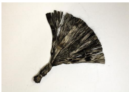
(a) Dry FRP anchor
