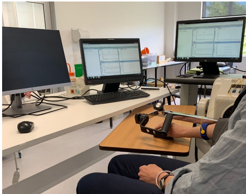
Figure 4.1: Experimental set up: Elbow flexor force was evaluated using a Biodex Multi-joint system. Participant sat upright with elbow-joint strapped to padded surface for upward elbow flexion. Screen placed directly in front of participant for force feedback. Shoulders and left knee were restrained by nylon straps to minimise shoulder and leg movement. An adjustable rolling table was placed directly under the restrained right arm for performance of the Fitts movement task. Table height was adjusted such that it allowed a swift swap between performance of the elbow flexion contraction and grasping the mouse for motor task performance.
