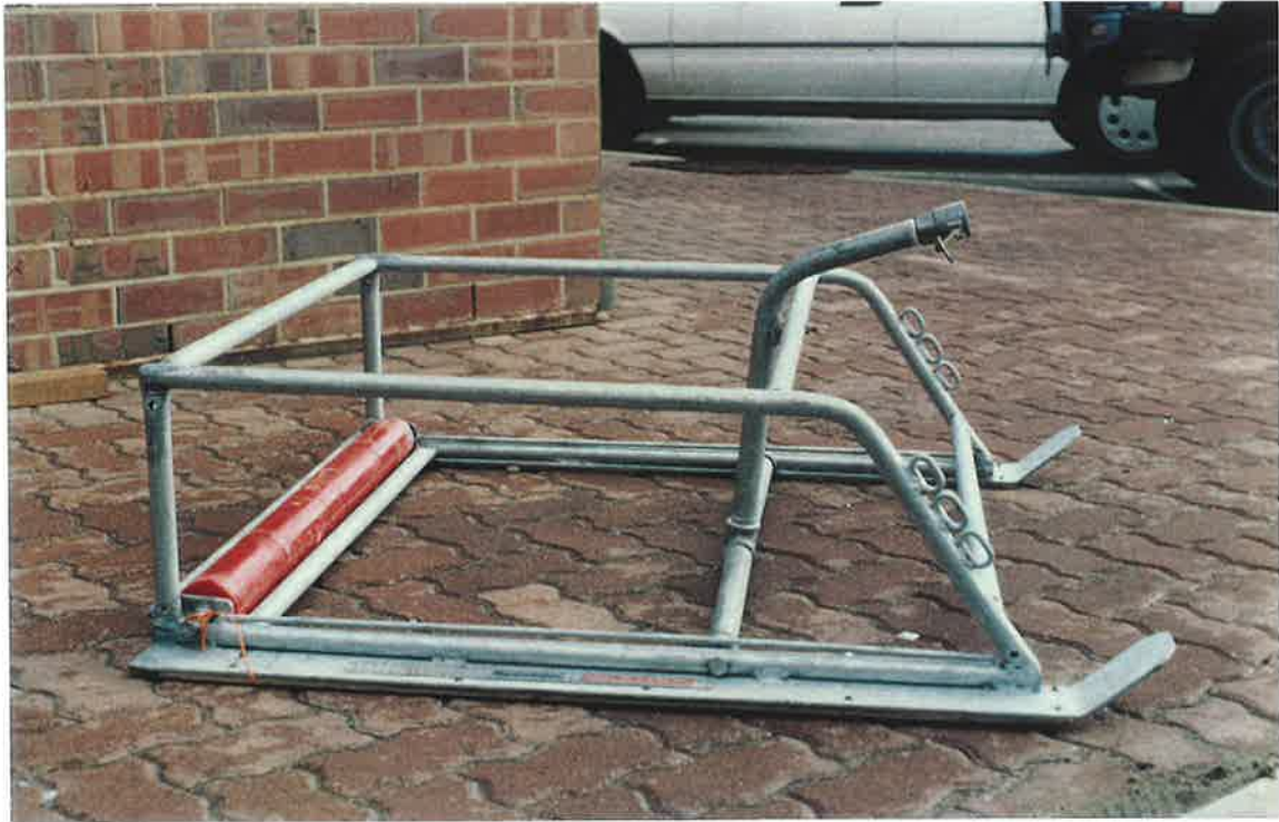
Plate 1 Jet net design showing the galvanised iron frame, skids and rollers. The dimension of the frame is 1.0 m wide and 0.95 m long with 100mm x 5mm skids lined with marine ply and rubber rollers at the back of the frame for ease of towing. The central vertical bar connects to the water hose.
