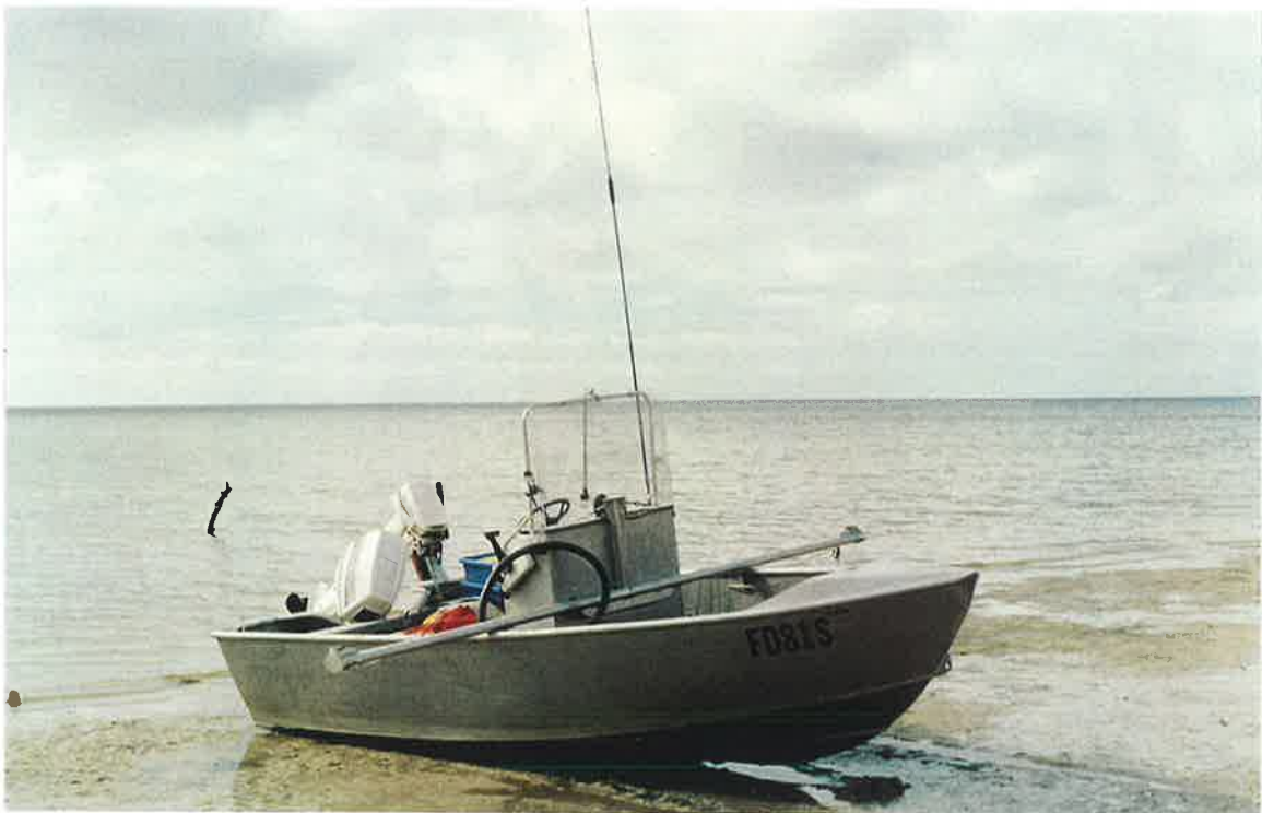
Plate 4 Boat used for sampling, shallow draft, 6m aluminium net boat with boom attached for towing. The net was towed approximately 5 metres behind boat to avoid prop wash at a speed of 1000 to 1600 rvs per minute depending on tidal movement. A 100 m 2 trawl was completed in two to three minutes.
