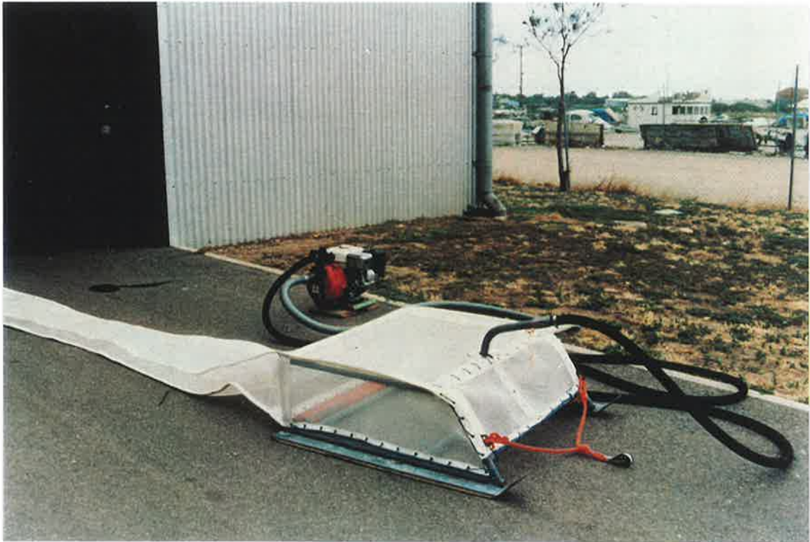
Plate 3 Jet net shows a fully closed net in front (2mm mesh), connected water hose and pump with intake hose. The bridle is used to connect to the hauling rope attached to boom on sampling boat.
