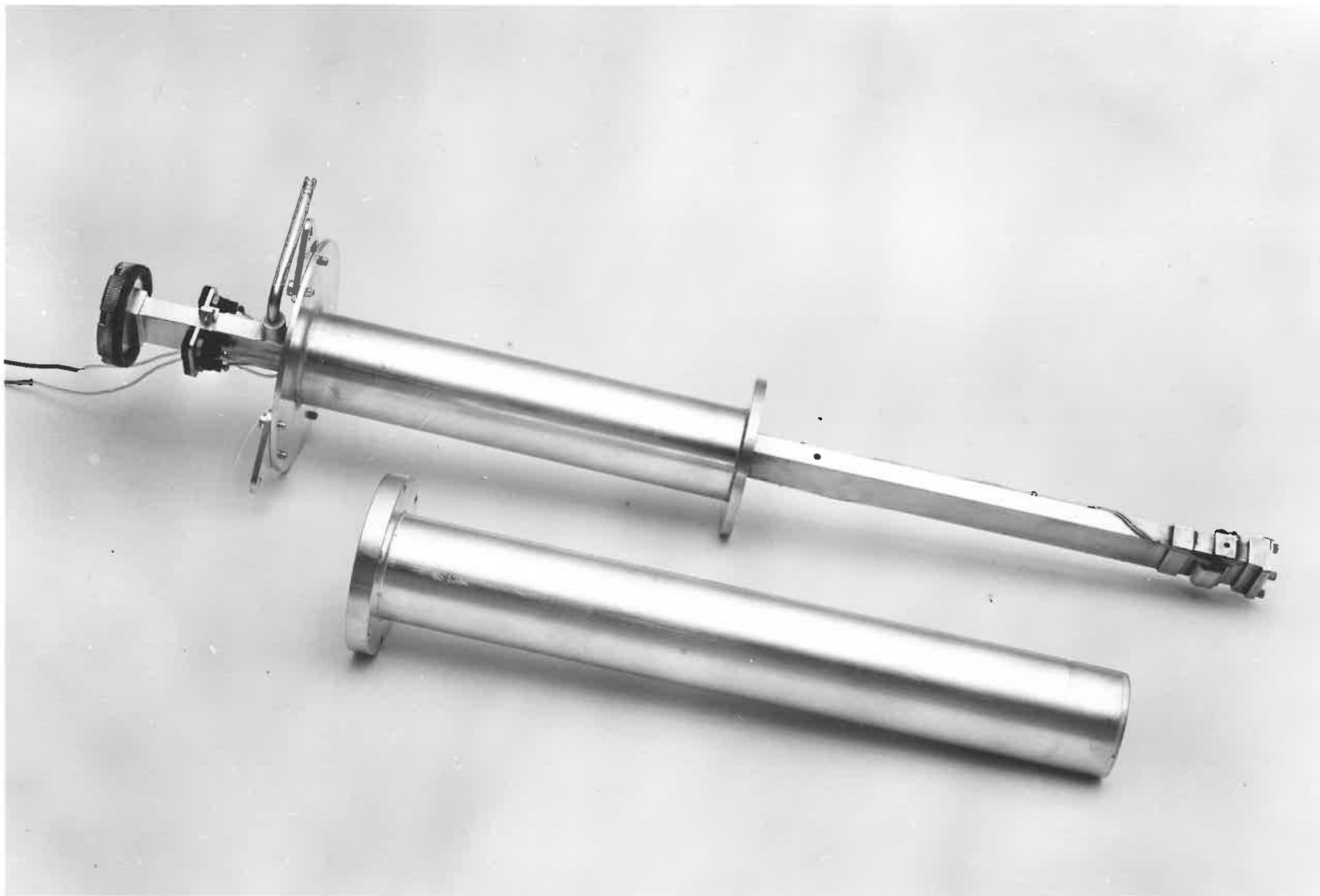
Fig.3.6 The High Temperature Cavity
