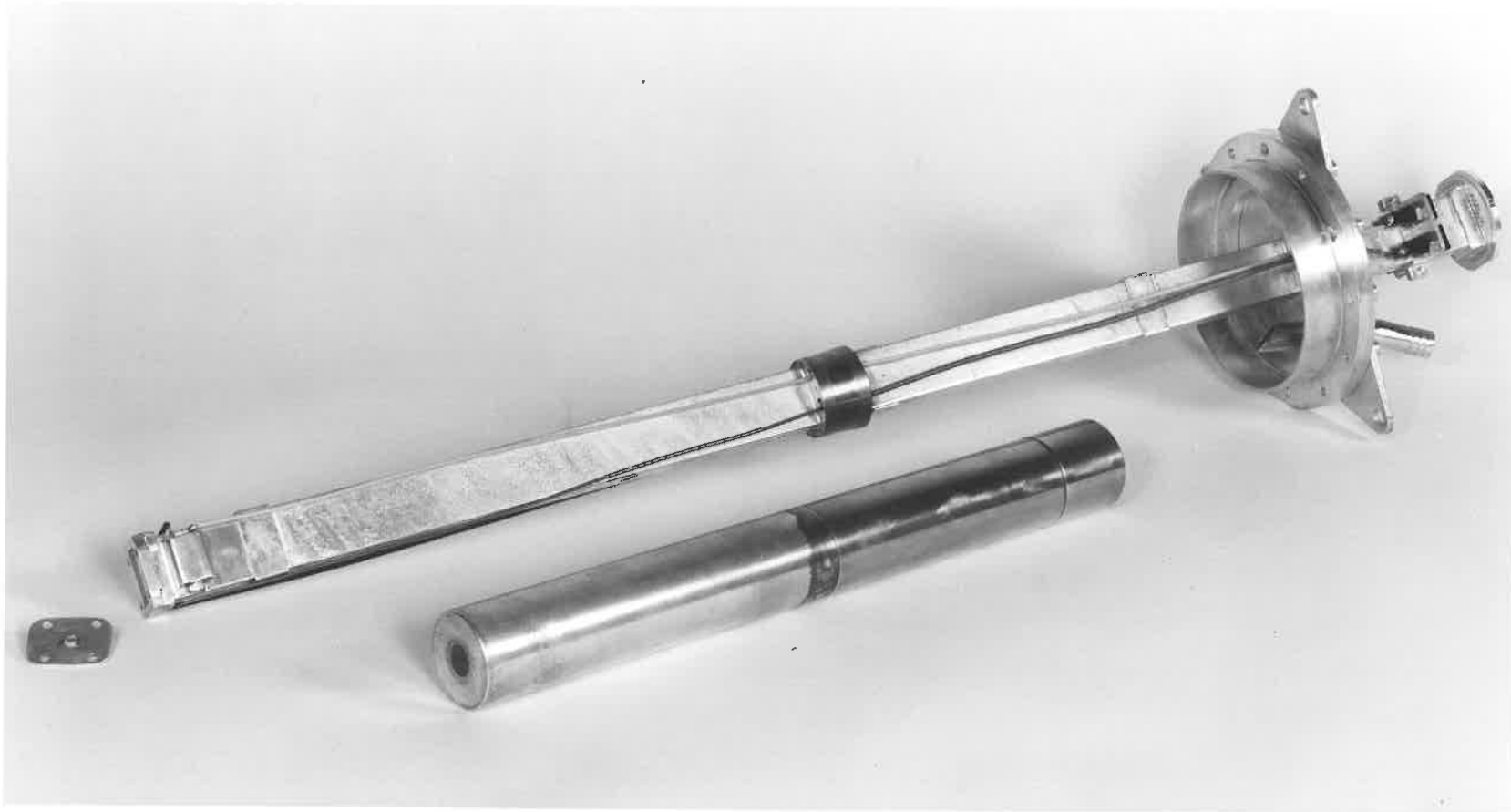
Fig.3.8 The Low Temperature Cavity
