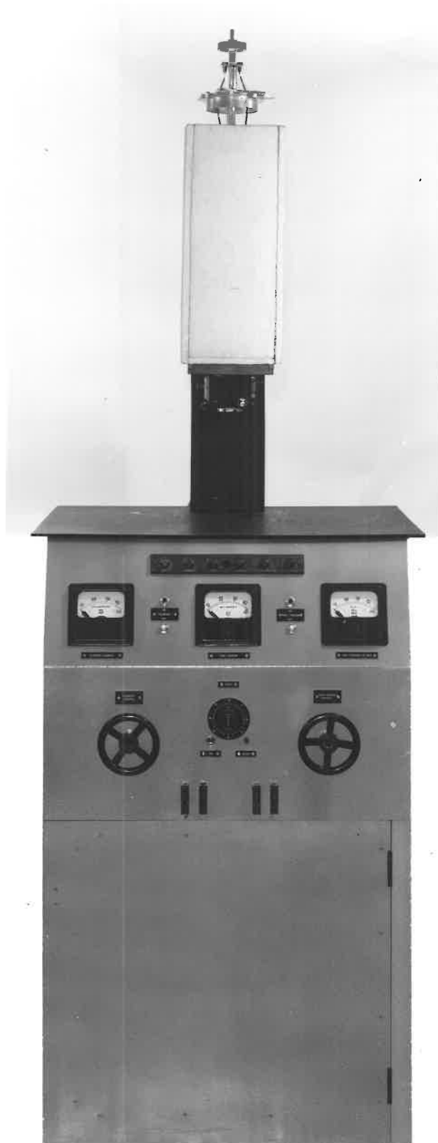
Fig.3.9 The Low Temperature Cavity Positioned on the X-ray Tube.
