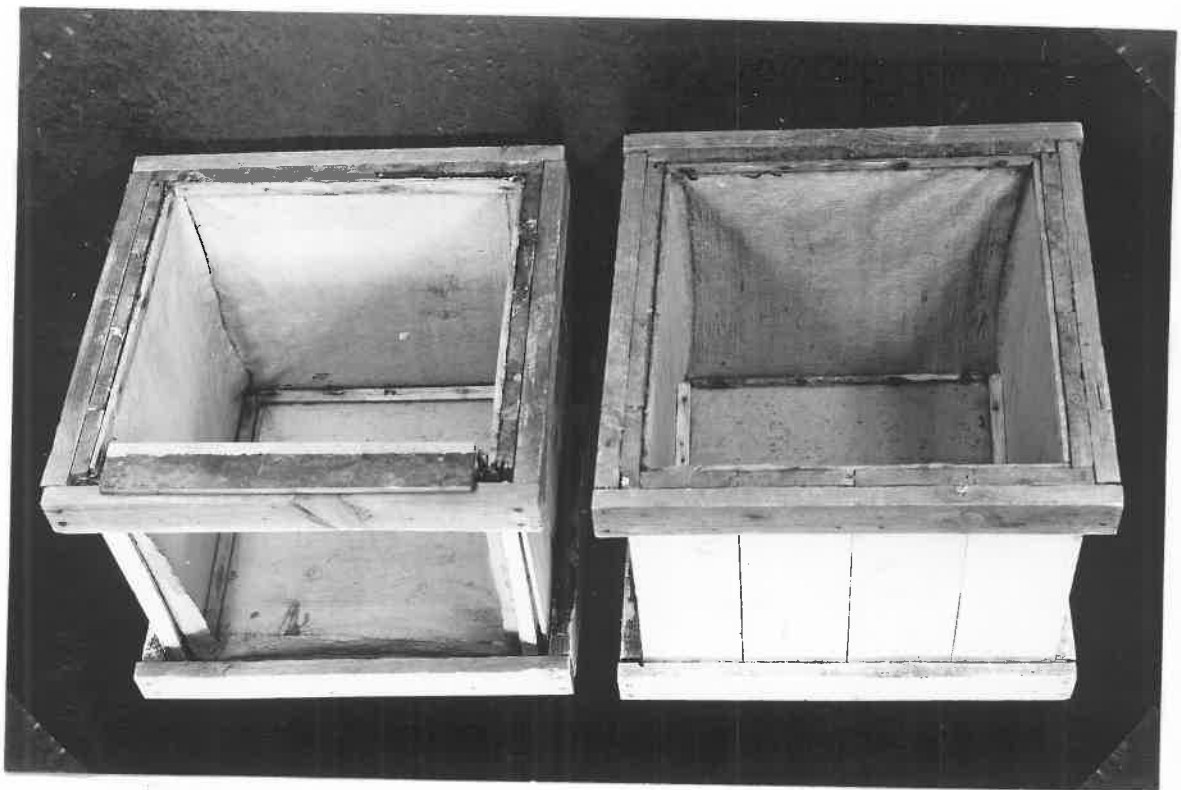
Plate 1. Wooden boxes used to control hours of daylight on cabbage plants grown in the field (Expt. 2).
