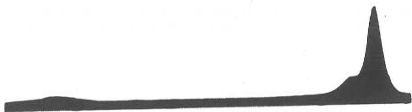
Fig. III-1. Electrophoretic pattern (ascending limb) of the ovalbumin complex at pH 8.7 0 in "Veronal" buffer, ionic strength 0.05, after three hours at a potential gradient of 6.2 volts/cm.
