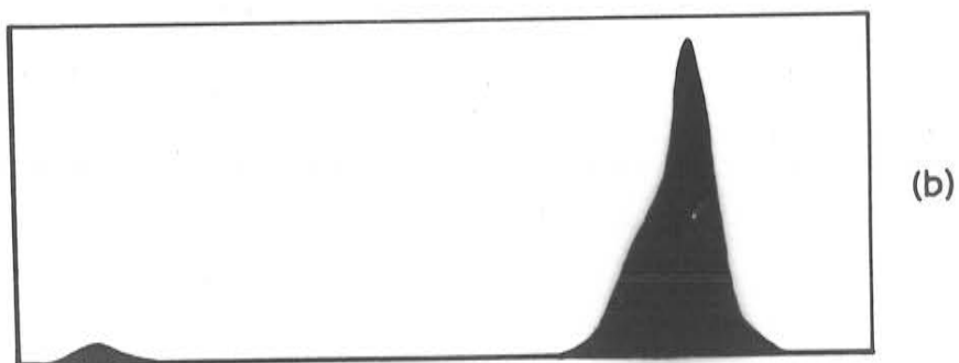
Fig. IV-3. Electrophoresis patterns (ascending limbs) of iodine-modified ovalbumin at pH 8.70 in "Veronal" buffer, ionic strength 0.05, after three hours at a potential gradient of 6.2 volts/cm.: (a) a freshly prepared sample; (b) a sample which had been stored for four months.
