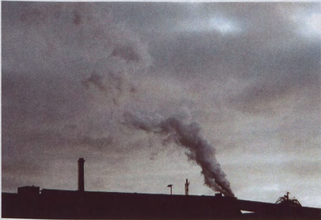
Figure 1-1 A typical example of an industrial jet in crossflow; the discharge of smoke into the atmosphere from a chimneystack (photo courtesy of Dr Gus Nathan).
