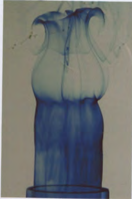
Figure 7-1 Jet shear layer development for a jet with zero crossflow at a jet Reynolds number of 4000.
