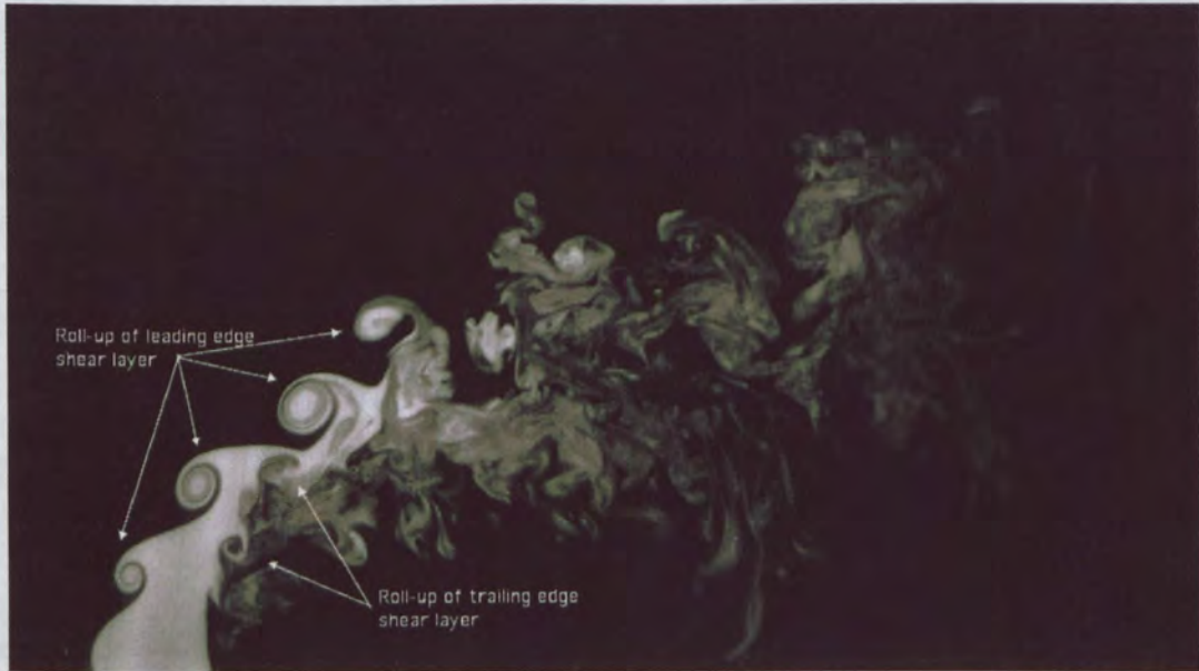
Figure 2-1 PLIF image along the jet axis of symmetry of a transverse jet, with a jet Reynolds number of 4000, at a velocity ratio of 2, showing a cross-section of the jet shear layer structures.
