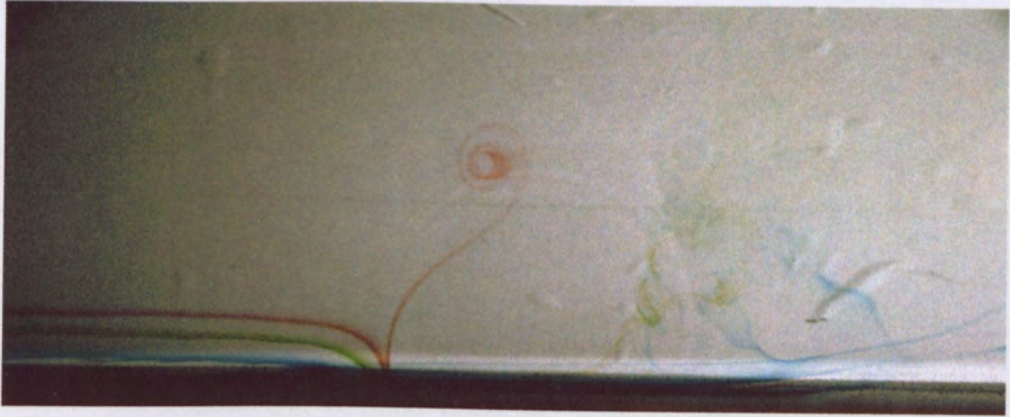
Figure 7-41 A false colour composite image composed from three separate images showing the path of dye introduced from different heights above the floor. R=4 , Re=2000 , \delta/d=0.3
