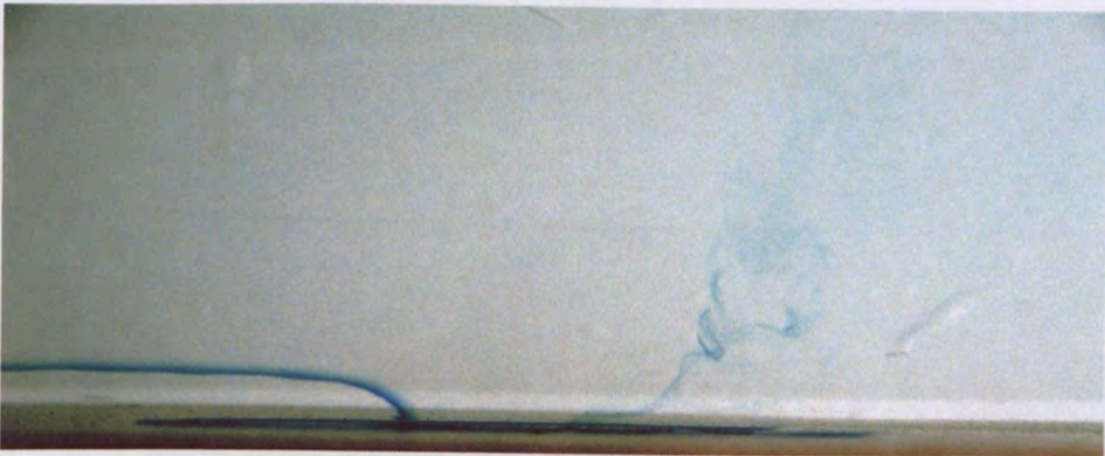
Figure 7-39 Image showing the path of dye introduced from an upstream location that impinges on the upstream corner of the jet pipe. Some dye then emerges bundled up with one of the counter-rotating vortices. R=4 , Re=2000 , \delta/d=0.3
