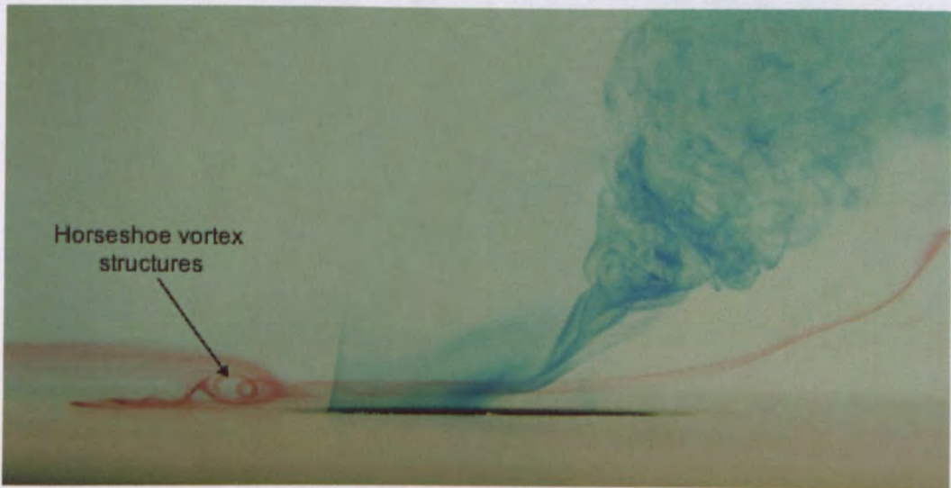
Figure 7-40 Dye visualisation showing the horseshoe vortex system shown with red dye. The jet shear layer is shown marked with blue dye. R=4 , Re=2000 , \delta/d=0.3
