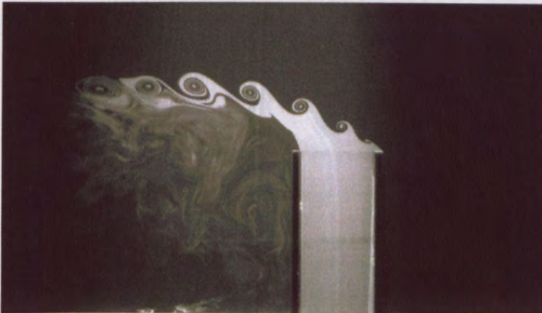
Figure 6-18 Instantaneous cross-section through the plane of symmetry of an elevated JICF at a velocity ratio of 0.5. Re=2000 , Re_j=1000
