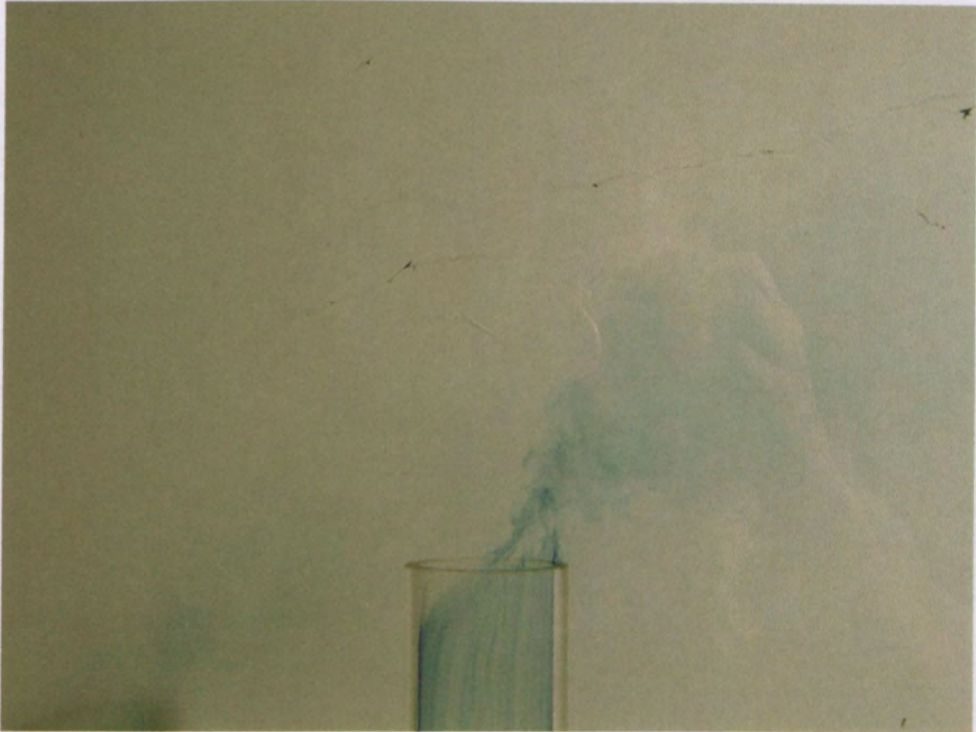
Figure 7-35 Comparison of the jet shear layer development at different Reynolds numbers for elevated jets at a velocity ratio of 4.
