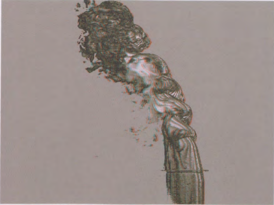
Figure 6-16 Volume rendering of the side view of an elevated JICF for a velocity ratio of 4.0. Re=2000 , Re_j=8000
