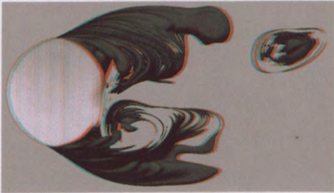
Figure 4-20 Red-blue stereo anaglyph, generated from volume renderings produced by T3D. This rendering was generated using an interpolation and over-sampling routine included in T3D. The renderings show a jet in crossflow (crossflow left to right, jet into page in top image, and out off page in bottom image). Thirty nine data planes were used to create the renderings, twenty of which were from images captured during the experiments, and 19 were produced during the processing of the data by interpolating the experimental data.
