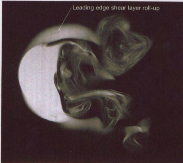
Figure 6-11 Single image slice from frame 7 of Figure 6-8 located 74mm (1.5d) above the jet exit plane.
