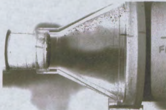
Figure 3-4 Dye visualisation of the flow through the wide-angle diffuser without the conical screen fitted. The flow appears to separate from the first corner of the diffuser as indicated by the dye and also the presence of the bubbles in the recirculation zone on the top inside surface of the diffuser.
