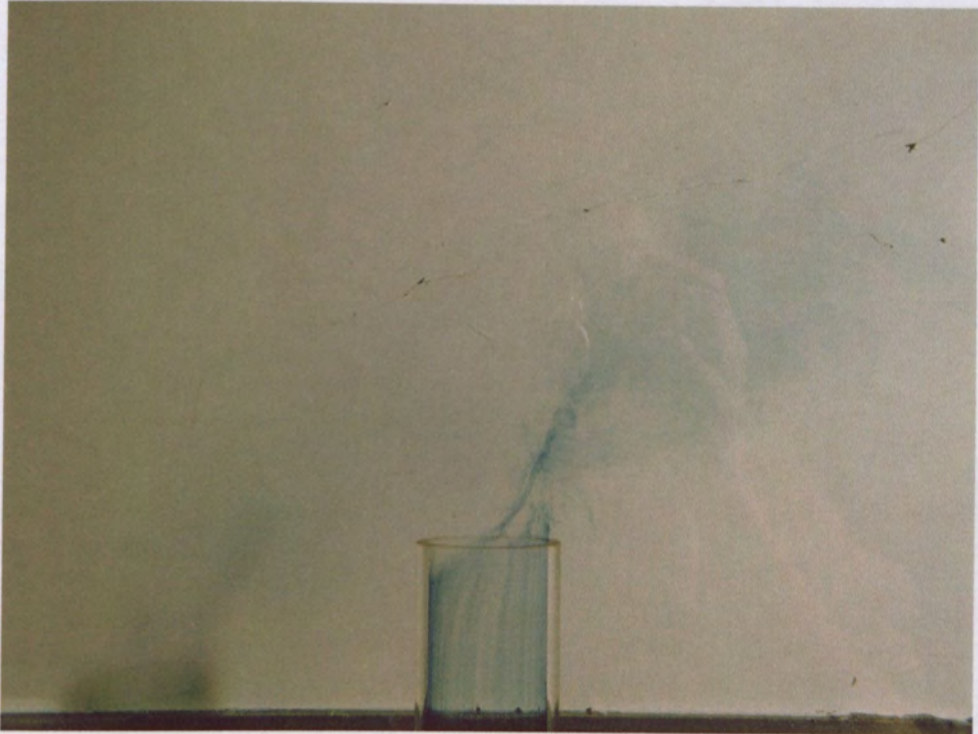
Figure 7-36 Comparison of the jet shear layer development at different Reynolds numbers for elevated jets at a velocity ratio of 6.
