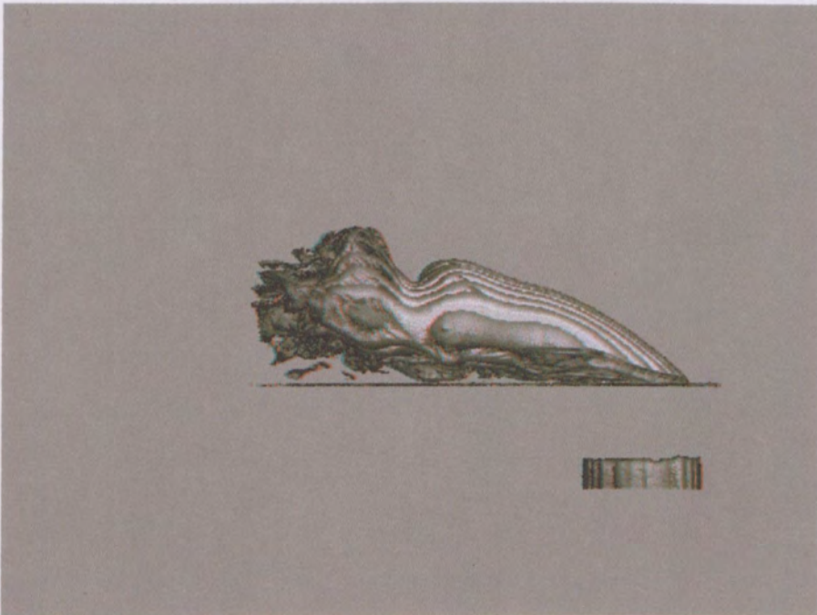
Figure 6-2 Volume rendering, shown as a red-blue anaglyph, of the side view of a flush-mounted JICF at a velocity ratio of 1.0. Re=2000 , Re_j=2000 , \delta/D=0.3
