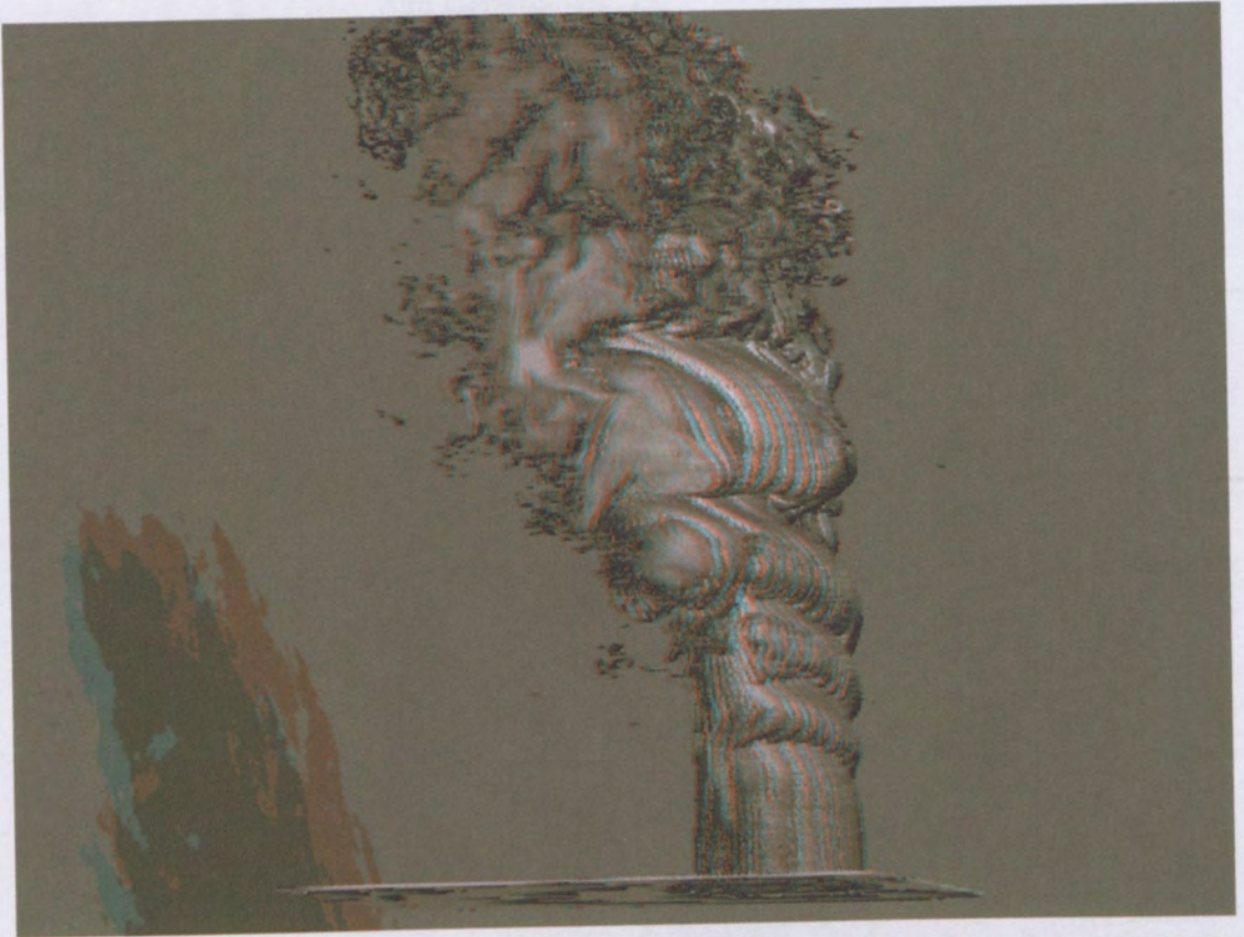
Figure 6-5 Volume rendering, shown as a red-blue anaglyph, of the side view of a flush-mounted JICF at a velocity ratio of 8.0. Re=1000 , Re_j=8000
