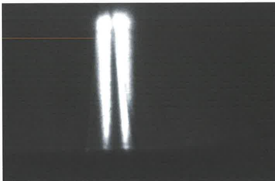
Figure 8: Uncorrected (50 shot average) Mode 1 OH PLPS image collected simultaneously with the PLIF image in Figure 7. The relative scale of the two flame images (the images in Figures 7 and 8 represent the full 378 x 576 array of the ICCD detector) indicates the relative resolution for the given experimental arrangement.
