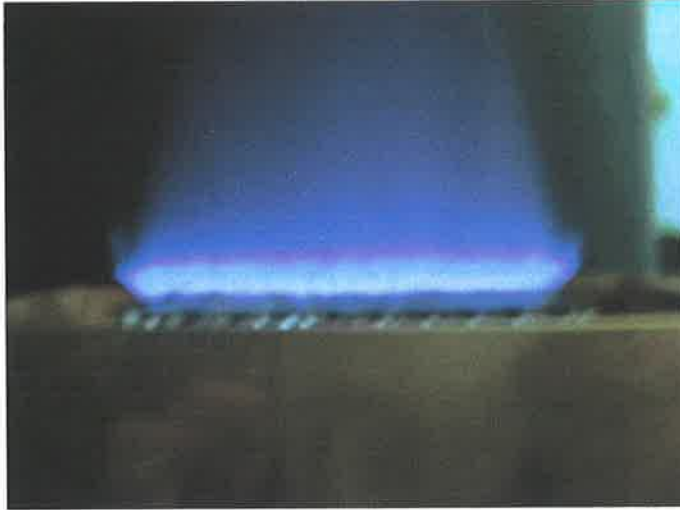
Figure 23: Near-stoichiometric natural gas/air flame lifted ~ 2-3 mm above the surface of the rectangular mixing burner.
