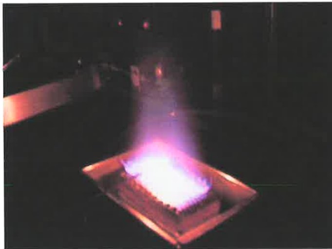
Figure 24: Rectangular mixing burner in operation. The nitrogen flow surrounds the \text{CH}_4 /air flame and isolates the combustion process from the ambient air.
