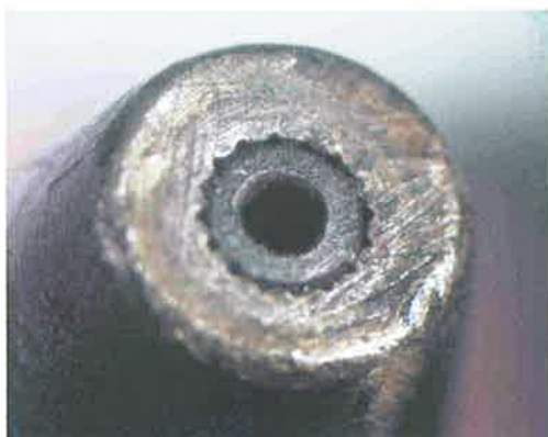
Figure 4: Tip of the modified glass-blowing burner used in the PLPS and PLIF imaging experiments. The tip of the torch has diameter 6.2 mm and the exit orifice has diameter 1.2 mm.
