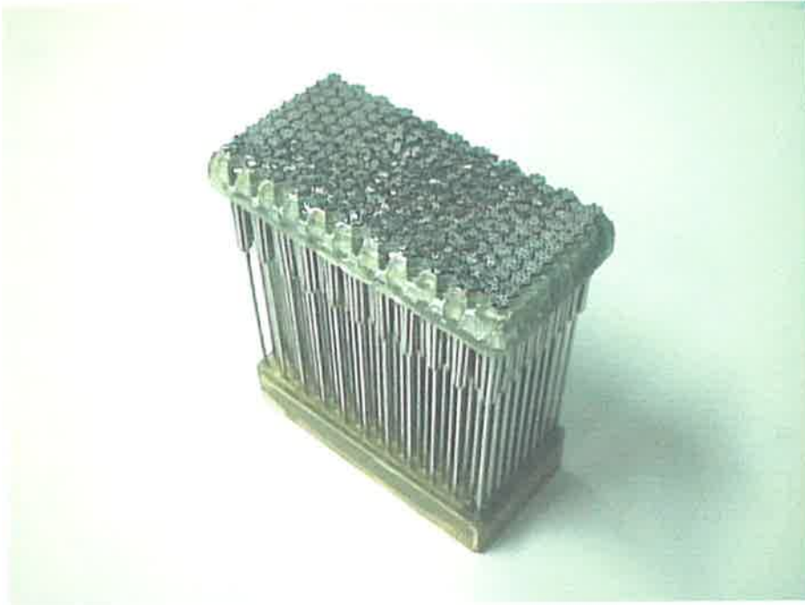
Figure 22: Fuel and oxidiser tube structure in the interior of the mixing burner. The shorter (0.6 mm internal diameter) tubes supply the air flow and surround the longer tubes supplying the natural gas. The internal tube structure was encased in a brass case and surrounded by a 18 mm wide nitrogen shroud.
