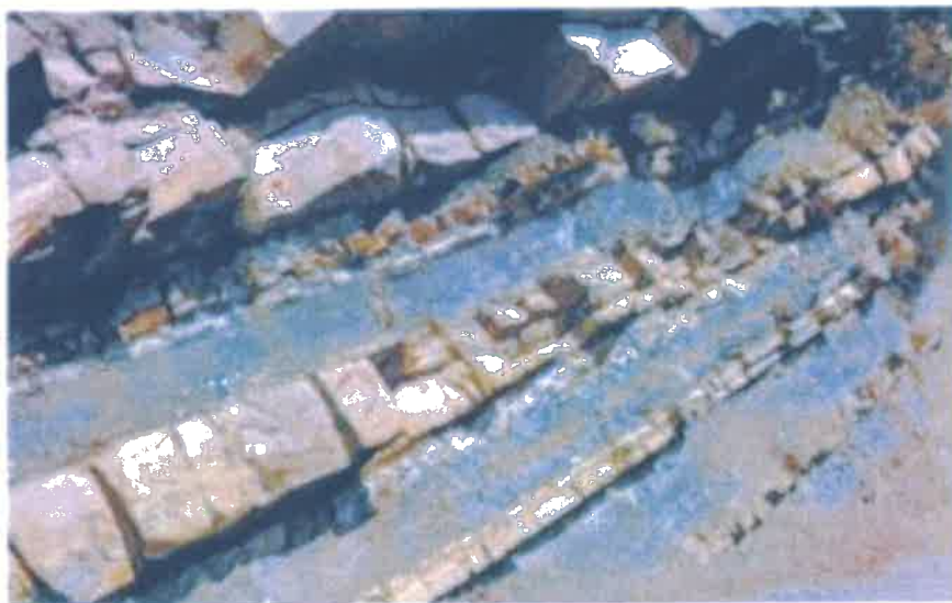
Figure 1.8. The effects of mechanical stratigraphy in a sandstone and shale sequence (~0.5 m thick). Fractures are well developed in the sandstone layers and poorly developed in the shale layers. Fractures within the sandstone layers are spaced proportional to bed thickness and terminate at bedding boundaries separating mechanical units (Golder, 2001).
