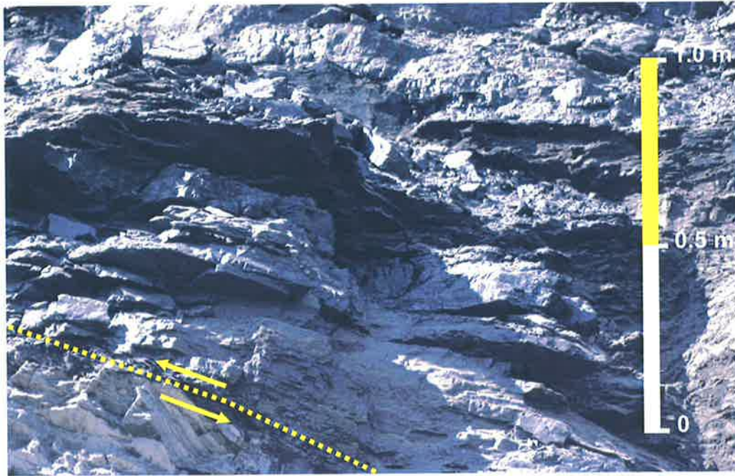
Figure 4.9. Thrust fault in highwall near ramp 2 with coal in the hangingwall (top right) and siltstone in the footwall (bottom left). The fault throw is not certain but is thought to be in the order of 1–3 m. The coal fabric has been overprinted with a foliation parallel to the fault ( 30^{\circ}\rightarrow 070^{\circ} ) in a damage zone approximately 1 m wide.
