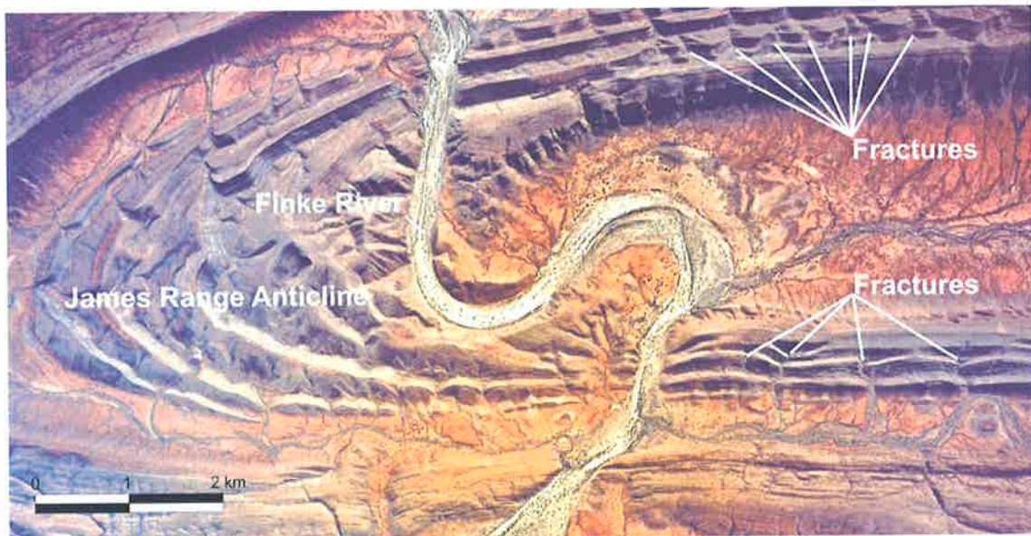
Figure 9.23. Aerial photographic expression of the regional fracture systems over the James Range Anticline. Note that the Finke River cuts through the anticline suggesting the contemporary drainage had established prior to folding.
