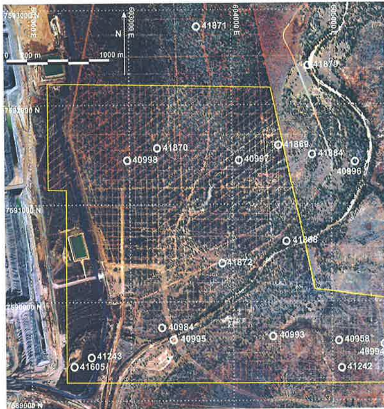
Figure 5.1. Location of 3D seismic survey (yellow outline) and boreholes with acoustic scanner image logs in the Goonyella Riverside underground area. The open cut mine is located to the immediate west.
