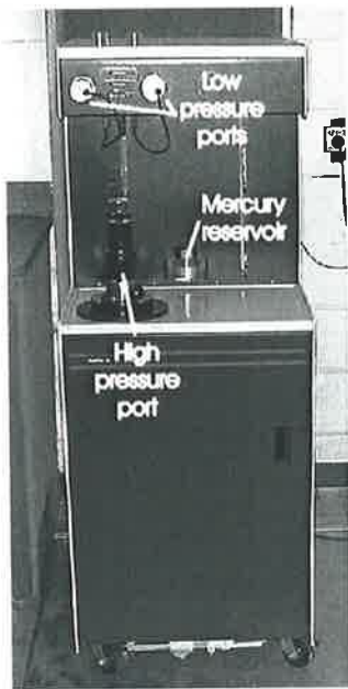
Left; the Micromeritics Autopore 9410 mercury injection porosimeter. Right; schematic view of an assembled penetrometer and the component parts (Bentley, 2000).
