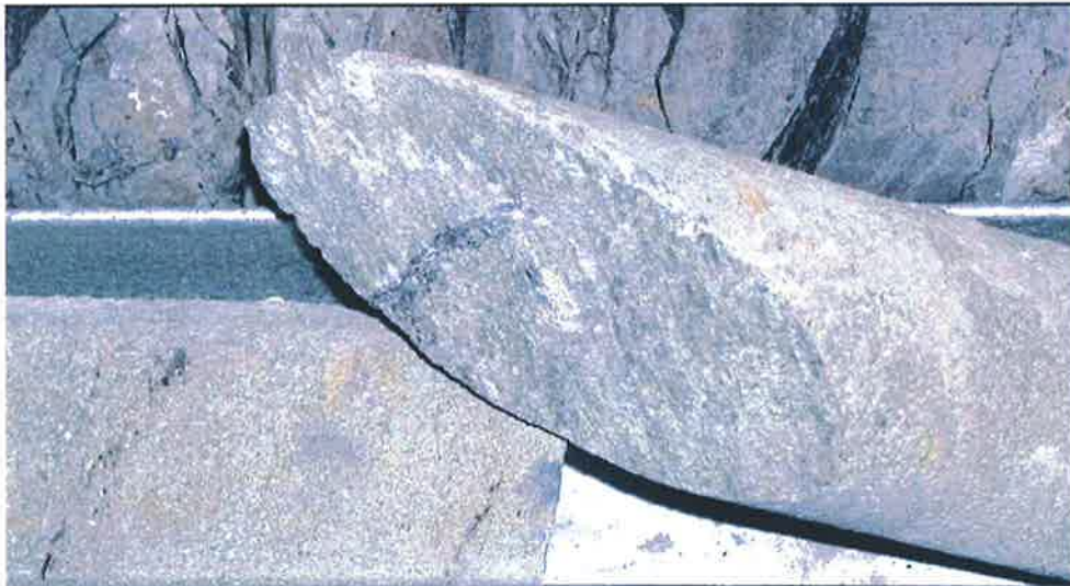
Figure 2.6. Shear fracture with slickensides, Scotia 4 (50 mm core).
