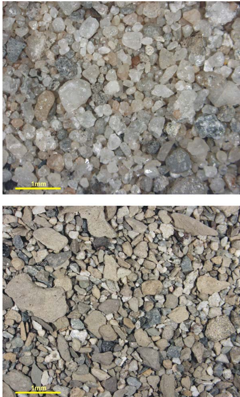
Figure 4.5 Photos from Windermere Sandstone Member cuttings showing its different character in two Otway Basin wells. A relatively well-sorted and well-rounded quartz-dominated coarse sandstone dominate in Trumpet-1 (top). In Diamond Swamp-1 (bottom), the Windermere consists of poorly sorted, sub-rounded pebbly feldspar-rich sandstone. Well locations are shown in Figure 4.6.
