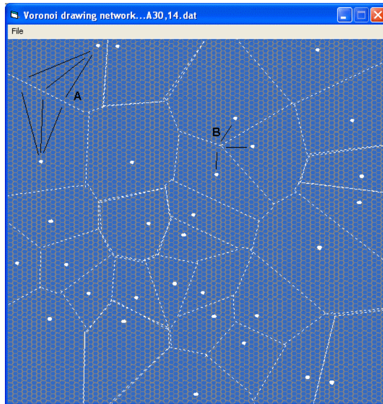
Figure 6.14: Output of the Voronoi drawing network is shown in white. The black lines at A show some binary symmetries that delineate the Voronoi segment. The black lines at B show a ternary symmetry that marks the point of intersection of Voronoi segments. (Some of the common segments are slightly disjoint due to the granularity of the distance measuring mechanism.)
