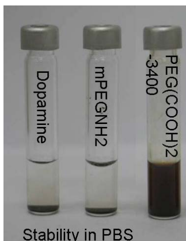
Figure 5-19: Stability of particles with dopamine coating (left), mPEG-NH 2 coating (middle) and PEG (3400) coating (right)
