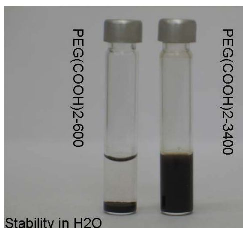
Figure 5-16: Stability of PEG (600) coating particles and PEG (3400) coating particles in MilliQ water
