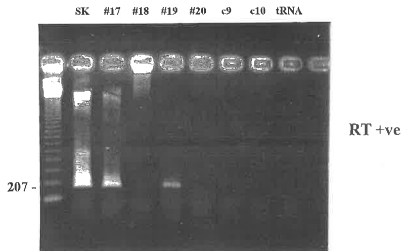
Figure 19. Single round RT/PCR (50 cycles) using inner tyrosinase primers on 2 ug RNA from 2 ml. whole blood samples from patients with known advanced/metastatic melanoma (#17 - #20). One 2 ml. sample of whole blood spiked with 10 SK 19 cells acted as the positive control, whilst 2 ml. samples of whole blood from healthy volunteers (c9, c10) and 1 ug. tRNA acted as negative controls. Detection of the 207 bp PCR product was seen in the positive control sample, the sample from patient 17 and the sample from patient 19. No false positive results were seen in any of the RT negative samples (results not shown).
