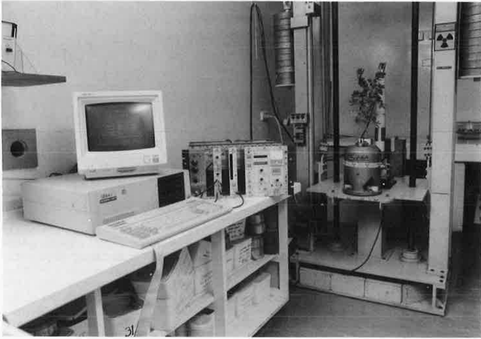
Fig. 1. Gamma scanning system with associated scalar and microcomputer control unit.
