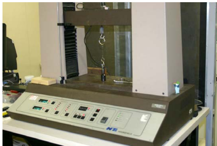
Figure 6: Force delivered by the coil springs was calibrated
