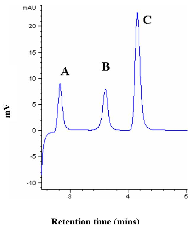
**Figure 4.1.** Separation of imazapyr (A), imazethapyr (B), and imazaquin (C) in mixed standards of  $1 \mu\text{g mL}^{-1}$  water by HPLC on a reverse phase  $\text{C}_{18}$  column.
