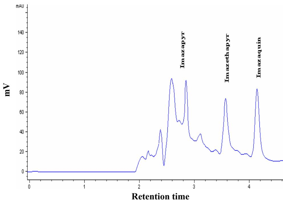
**Figure 3.6.** Chromatogram of spiked soil sample ( $1 \mu\text{g g}^{-1}$ ) after passing the soil extract through a  $\text{C}_{18}$  and then a SCX cartridge.
