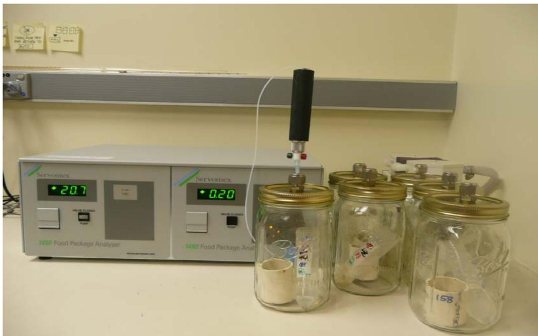
**Figure 5.2.** Image of infra-red gas analyser with the standard jars used in this study to measure CO<sub>2</sub>.
