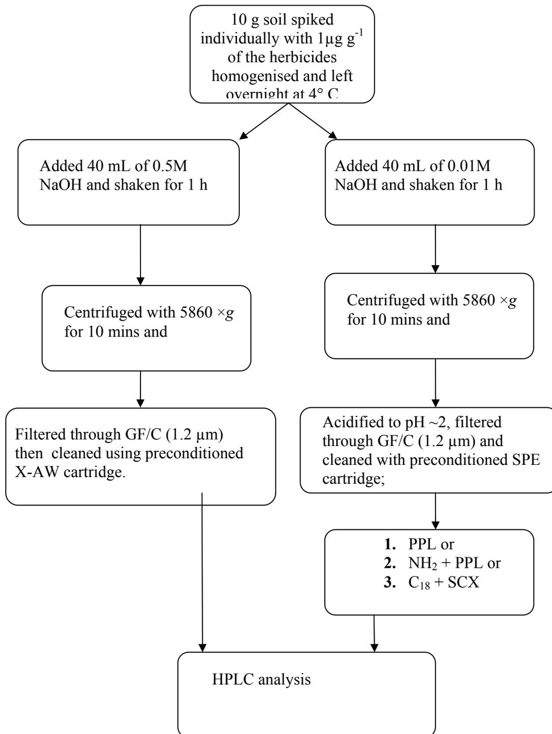
**Figure 3.1.** Flow chart of methodology for the extraction of imidazolinone herbicides from soil using different SPE cartridges.
