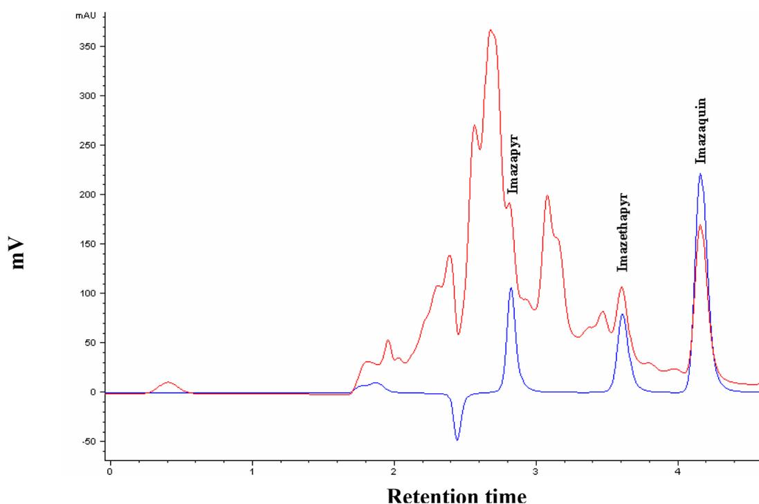
**Figure 3.5.** Chromatogram of imazapyr, imazethapyr and imazaquin in a standard solution ( $10\mu\text{g mL}^{-1}$ ) (blue line) and in a 0.5M NaOH soil extract passed through a PPL cartridge (red line).
