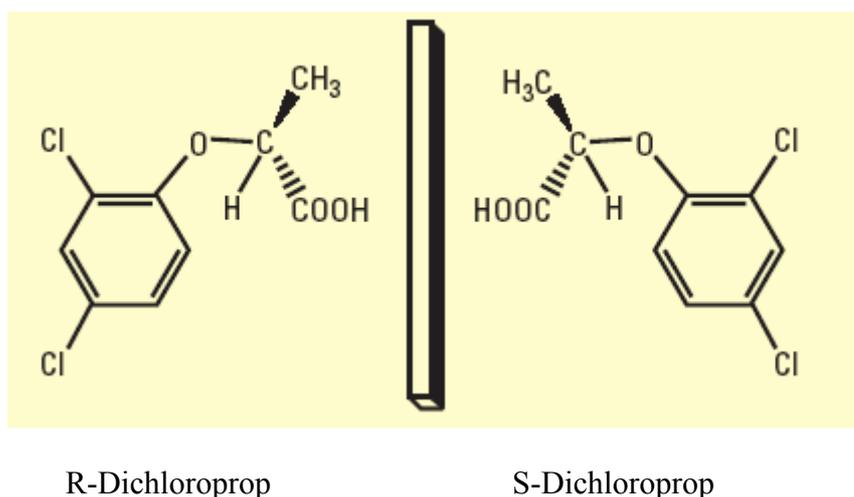
**Figure 2.4.** Two enantiomers (mirror image isomers) of dichloroprop (Garrison et al., 1996).
