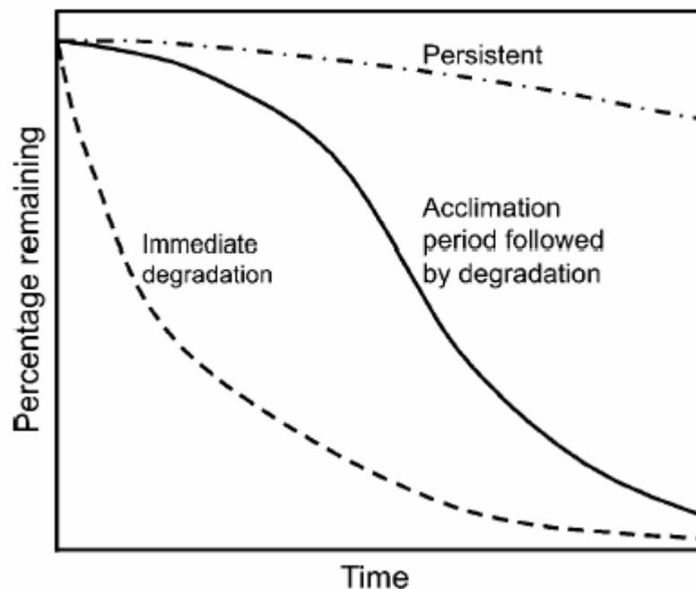
**Figure 2.2.** Different types of microbial degradation of pesticides.
