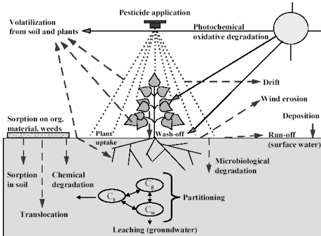
**Figure 2.1.** The main processes influencing the behaviour of pesticides in the environment.  $C_g$ ,  $C_w$  and  $C_s$  represent the pesticide concentrations in the gas, aqueous and solid phases, respectively (Wolters et al., 2004).
