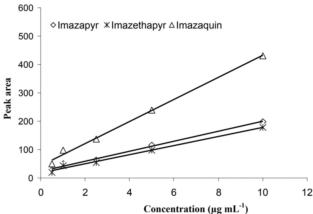
**Figure 3.2.** Calibration curves for imazapyr, imazethapyr and imazaquin at the concentration level of 0.5 to 10  $\mu\text{g mL}^{-1}$ .
