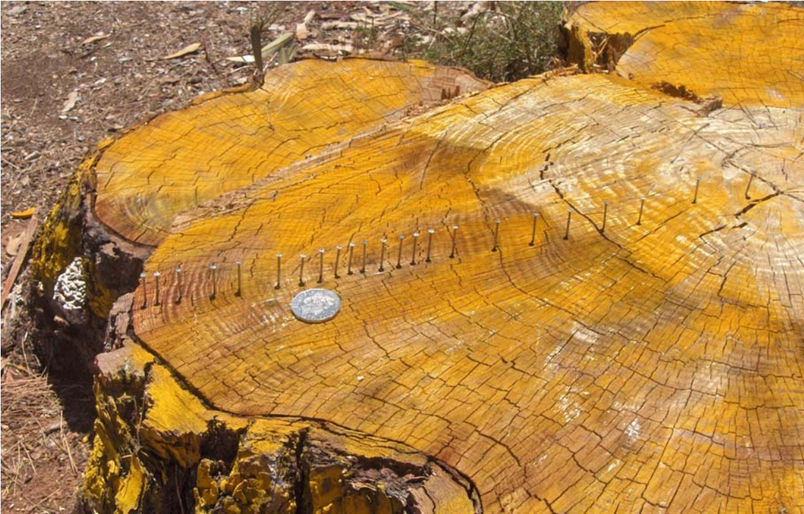
Figure 7.7. Photograph of growth ring counting on felled tree stump in Park 17. Each steel pin denoted five growth rings, and are shown here to scale with a Commonwealth of Australia 50-cent piece.
