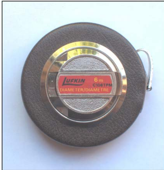
Figure 7.3. (Above) Lufkin Artisan Diameter Tape C106TPM. The Diameter Tape casing itself, shown here, is 8.5 cm in diameter.
