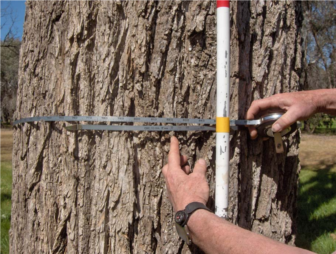
Figure 7.5. Measuring trunk DBH using the Lufkin Artisan Diameter Tree Tape. DBH was measured at 1.3m above ground level, as indicated by yellow tape on the height measuring staff. This specimen had a DBH recorded of 82cm.
