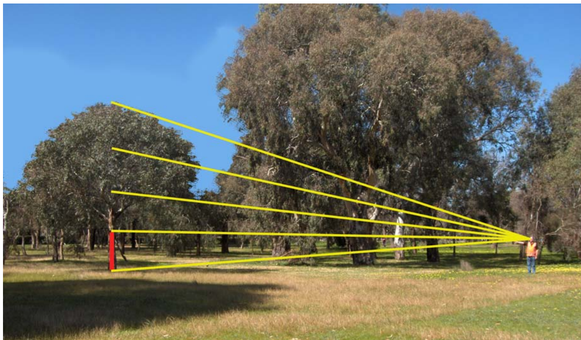
Figure 7.6. Measuring tree height in the field using the height measuring staff. The two-metre staff has been highlighted in red, with two-metre height measurements highlighted in yellow.
