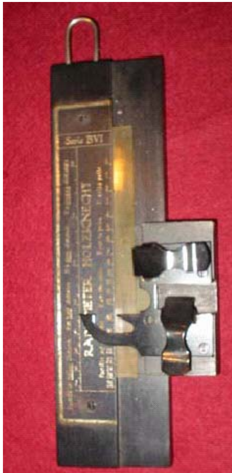
Figure 2.3 The Holz knecht chromoradiometer scale (Photograph courtesy of the Radiology Museum Brussels, Belgium)
