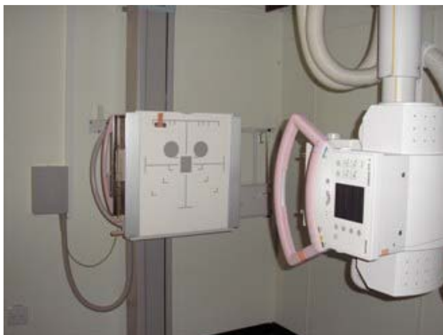
Figure 2.6 X-ray machine erect Bucky (centre left of photo) showing the physical arrangement of the three ionisation chambers used as x-ray detectors for the AEC.
