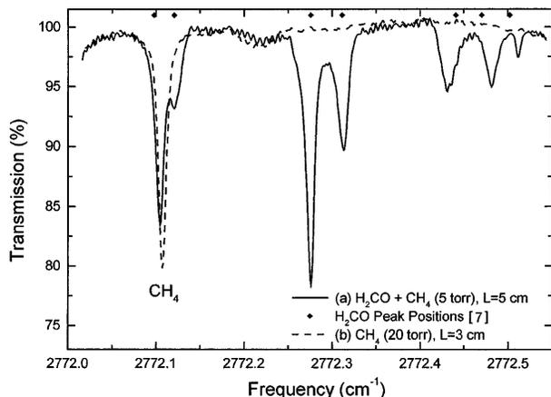
Fig. 4. Absorption spectra near  $2772.3 \text{ cm}^{-1}$  of (a) a  $\text{CH}_4$  and  $\text{H}_2\text{CO}$  mixture and (b)  $\text{CH}_4$ . The  $\text{H}_2\text{CO}$  peak were predicted in Ref. 7.
