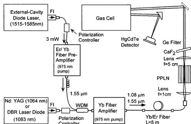
Fig. 1. Schematic of the dual-wavelength amplifier-pumped DFG source-based gas sensor: FTs, Faraday isolators.
