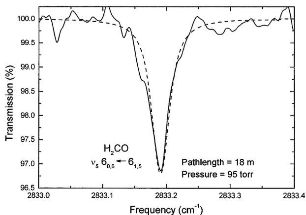
Fig. 5. Absorption spectrum of the  $\nu_5$   $6_{0,6} \leftarrow 6_{1,5}$  transition at  $2833.2 \text{ cm}^{-1}$  for a calibrated 5.78-ppm  $\text{H}_2\text{CO}$ -in- $\text{N}_2$  mixture. A Hitran 96 spectrum of 5.78-ppm  $\text{H}_2\text{CO}$  is shown for comparison.
