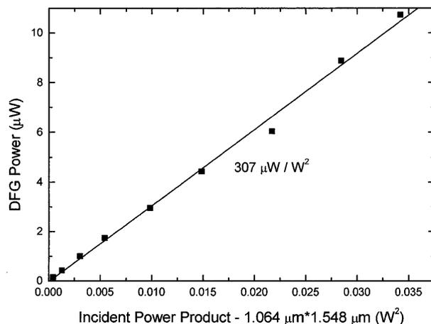
Fig. 3. DFG power at 3.4  $\mu\text{m}$  versus pump power mixing product  $P_{1064\text{ nm}} \times P_{1550\text{ nm}}$  for a 2-cm PPLN crystal.
