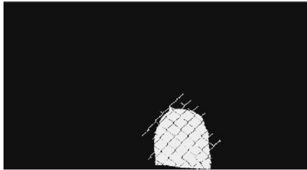
Fig. 7.18 The result of searching a big object in the binary image
