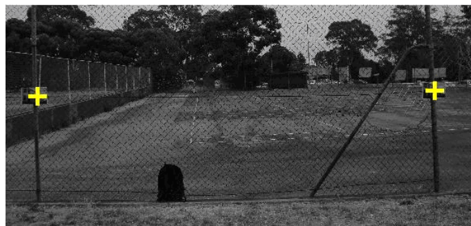
Fig. 4.13 Two CPs are automatically extracted from left and right posts of the wire fence with a template-based matching approach by using the SIFT operator in the AOI1_RI
