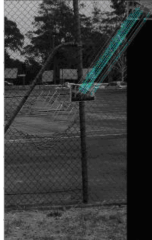
Fig. 4.12 The SIFT operator extracts 23 matched keypoints from the template_RI and region IV of the AOI1_RI
