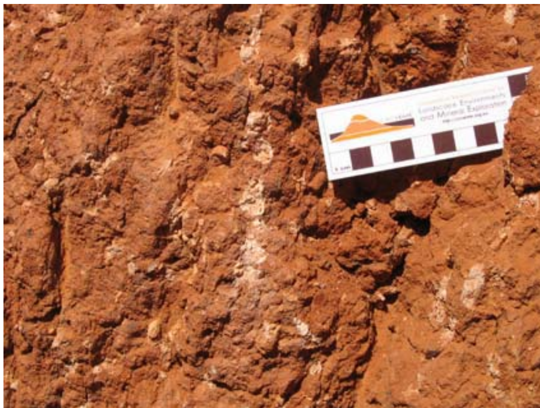
Figure 6.5: Rhizomorph and powdery nodule morphologies of regolith carbonates present in the Bk horizon.
