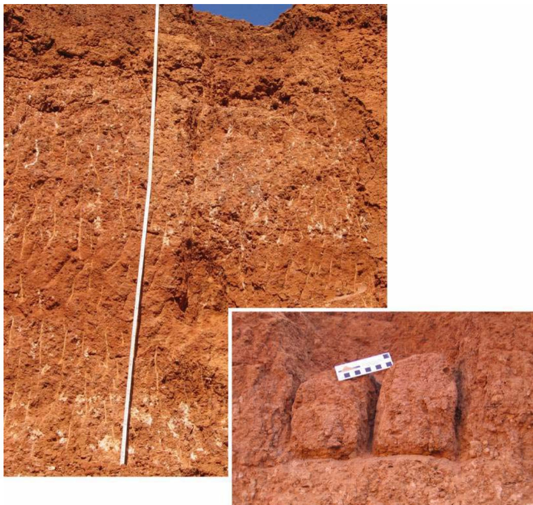
Figure 3.1: A prepared profile ready for sampling and undisturbed sample collection, White Dam Profile 1, Curnamona Province, SA (Profile depth ~ 2.3 m, inset scale bar 10 cm).
