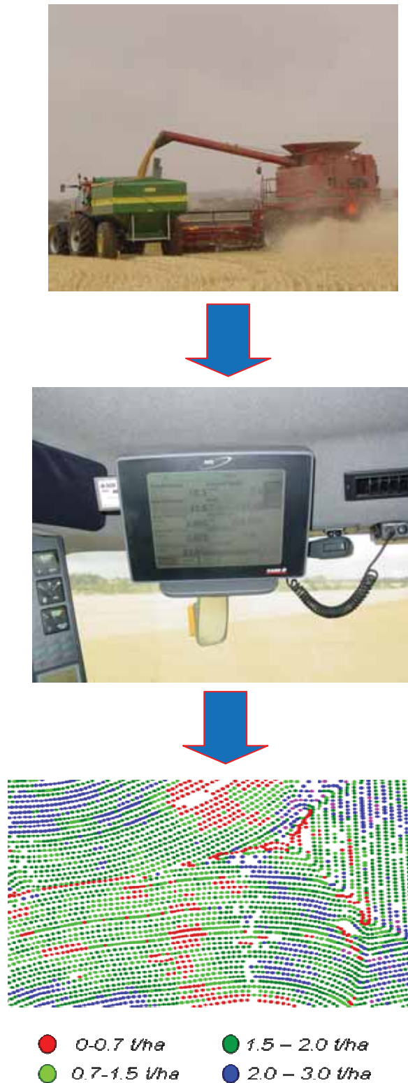
Figure 3 The yield mapping process: As the combine harvester harvests (a) data is collected to determine yield and the position of the harvester by the yield monitor (b). This process enables the two dimensional mapping of yield to identify its spatial variation within a field.
