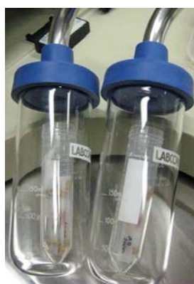
(b) Vacuum vials used in manifold drying; test tubes containing biotissue samples are clearly visible
