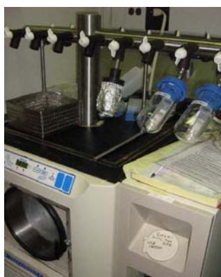
(a) The Virtis Freezemobile 25EL lyophiliser used in this study
