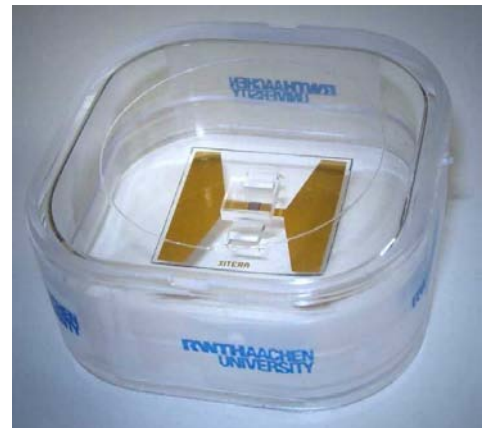
(b) PCA with bow-tie structure
