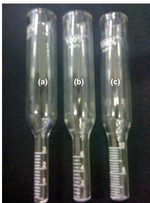
Figure 7.20: Spin test tubes for maximum (a) 3%, (b) 6%, and (c) 10% solids content
