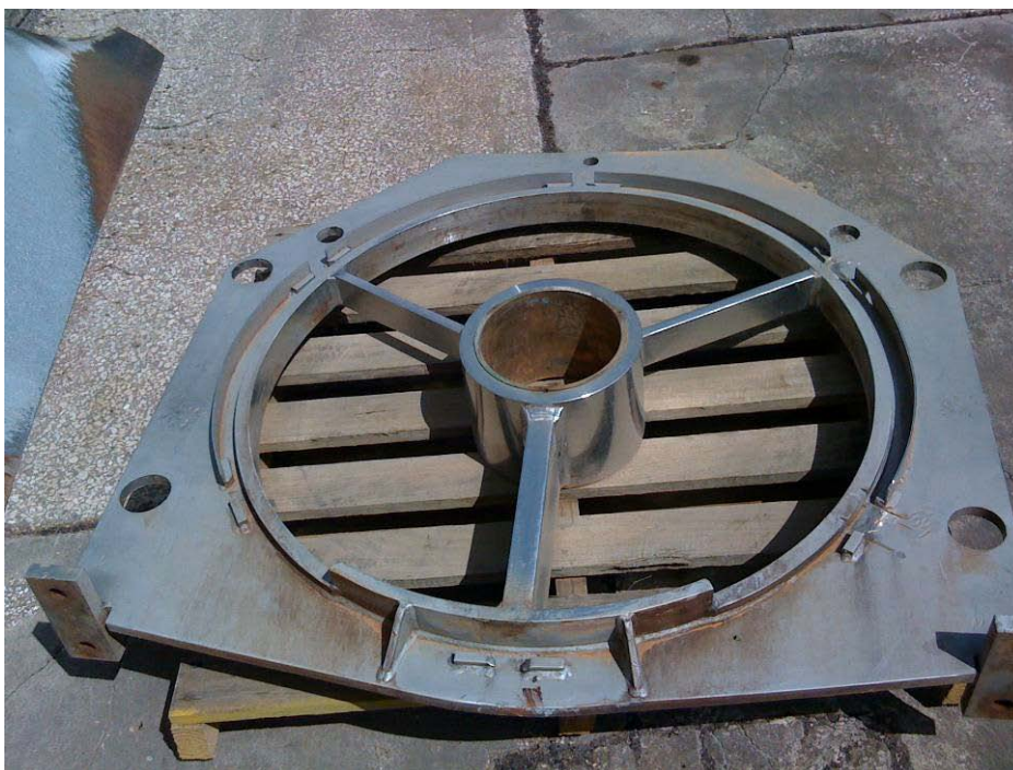
Figure 5.33: Anti-return device of Marzola PAP1000 continuous screw press
