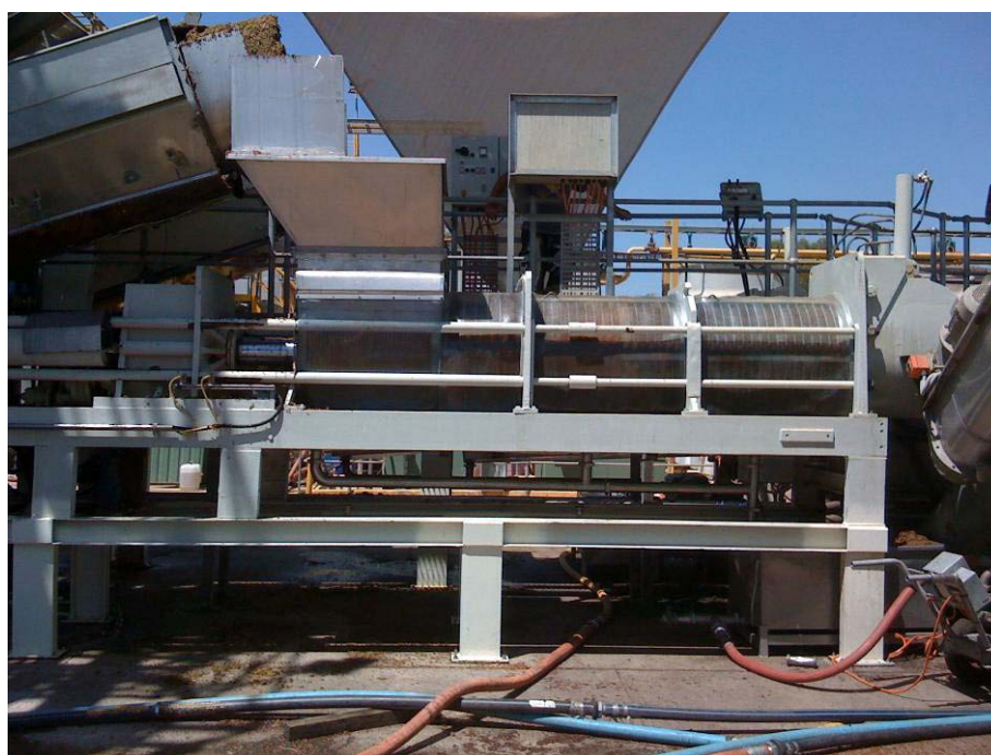
Figure 7.11: Coq 800 mm Bi-valve continuous screw press
