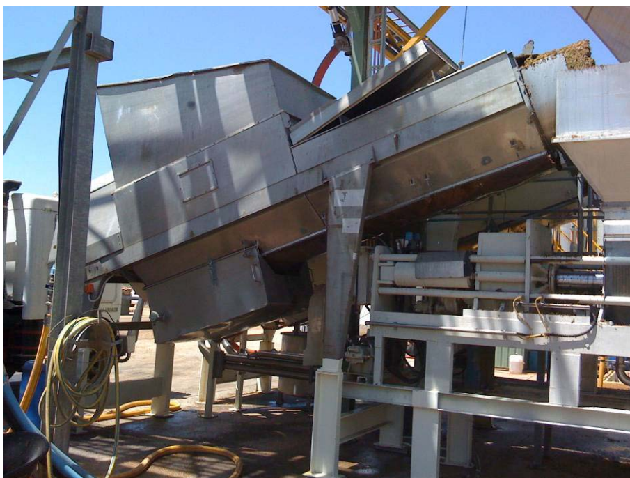
Figure 7.8: Miller 800 mm inclined drainer
