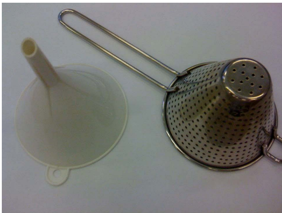
Figure 7.19: Stainless steel strainer and PP funnel for preliminary bulk solids removal
