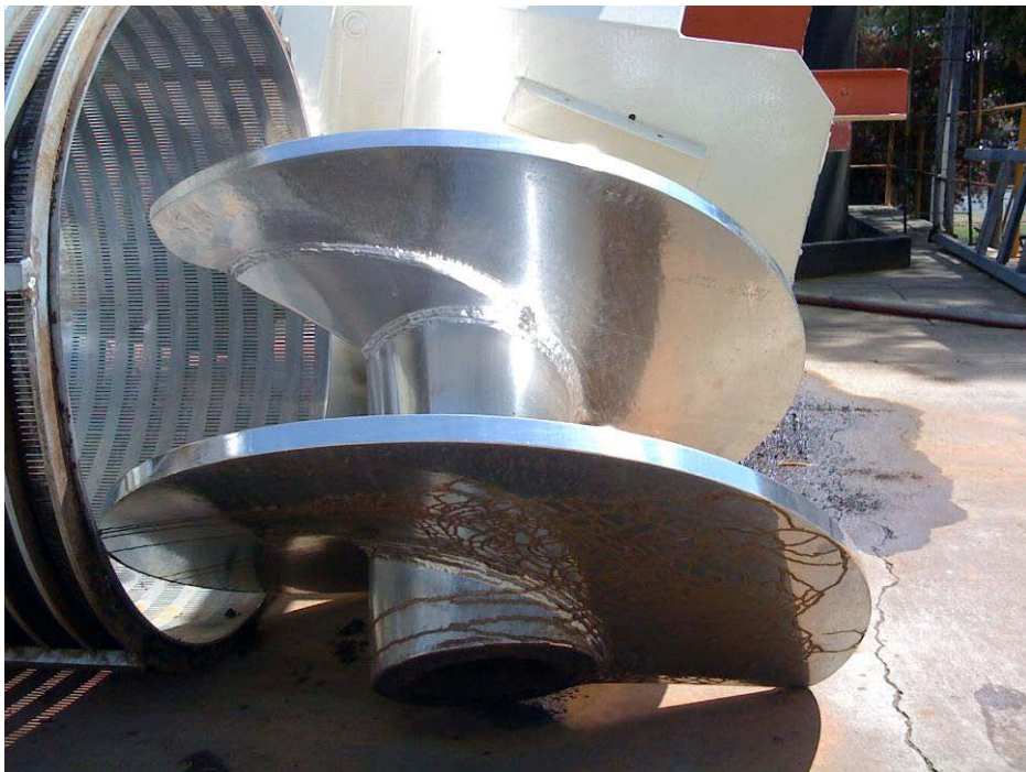
Figure 5.32: Second screw section of Marzola PAP1000 continuous screw press
