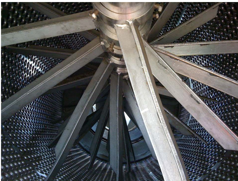
Figure 4.1: Destemmer paddles (view from stem-exit end)
