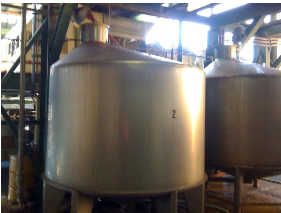
Figure 7.15: Two of the buffer tanks into which static drainer juice or membrane press juice flows
