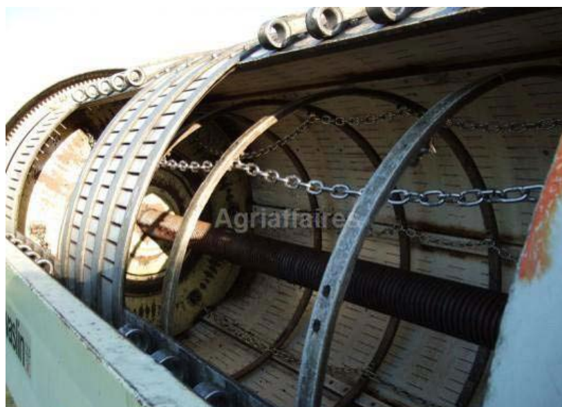
Figure 5.7: Rings and chains in a Vaslin 3.2 m 3 press (From: Agriaffaires.co.uk 2010)
