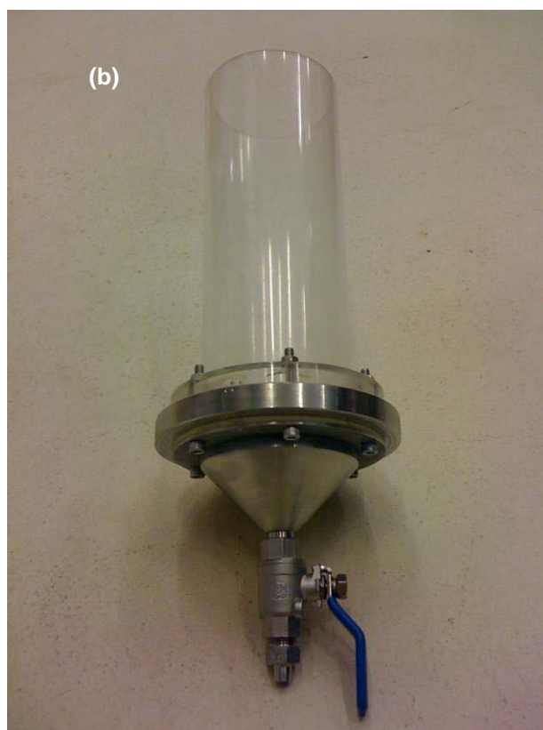
Figure 9.3: Laboratory pressing apparatus (a) mount, and (b) compression cylinder
