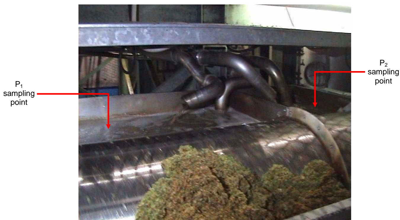
Figure 7.18: Rotary screens servicing 2 screw presses (Winery B - Process 1 sampling locations marked)
