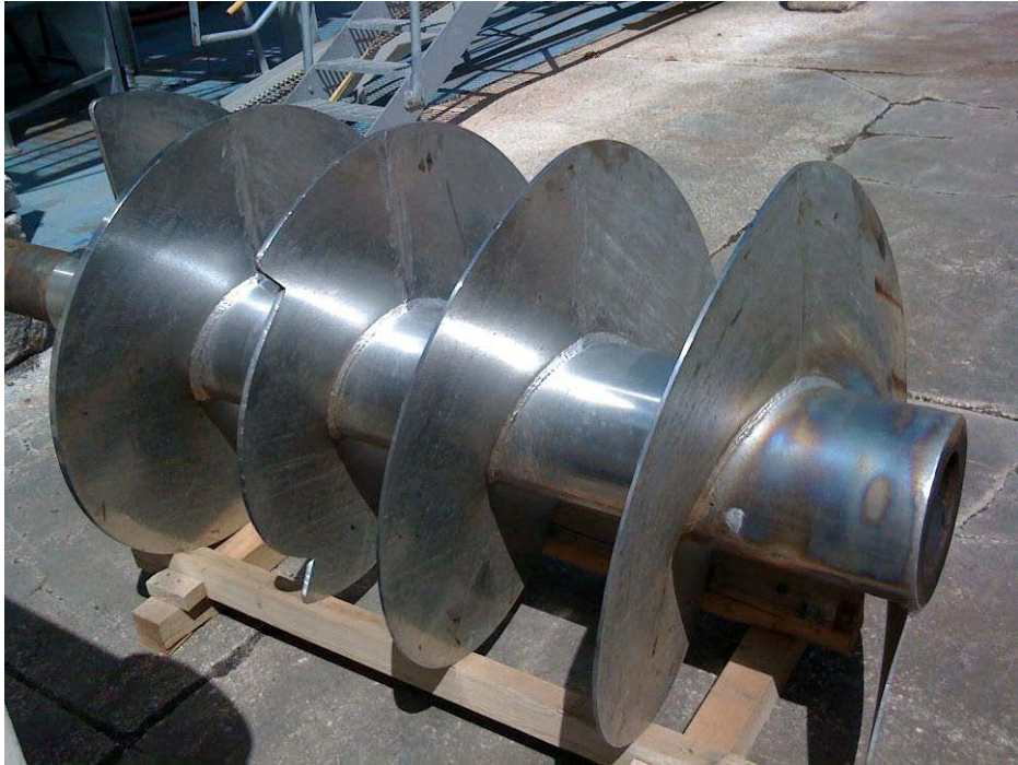
Figure 5.31: First screw section of Marzola PAP1000 continuous screw press
