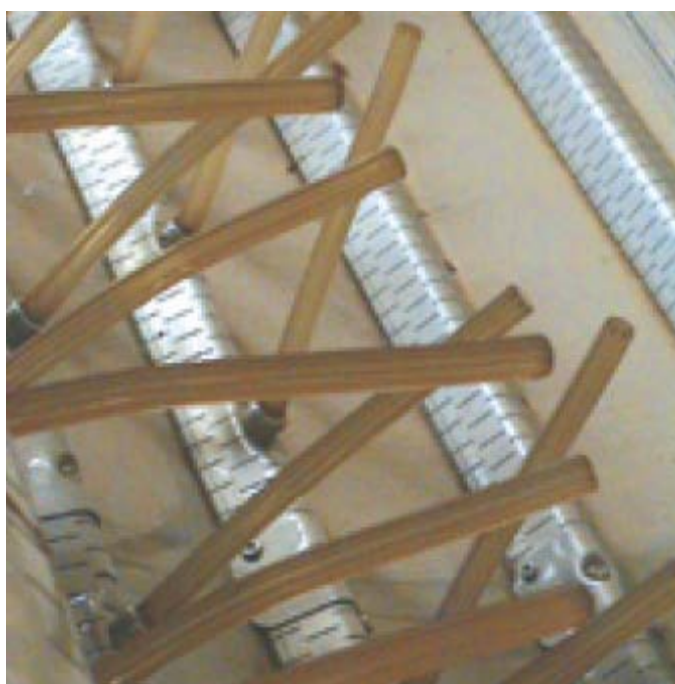
Figure 5.17: Three-dimensional drainage system for Bucher-(Vaslin) presses (From: Bucher-Vaslin 2010b)
