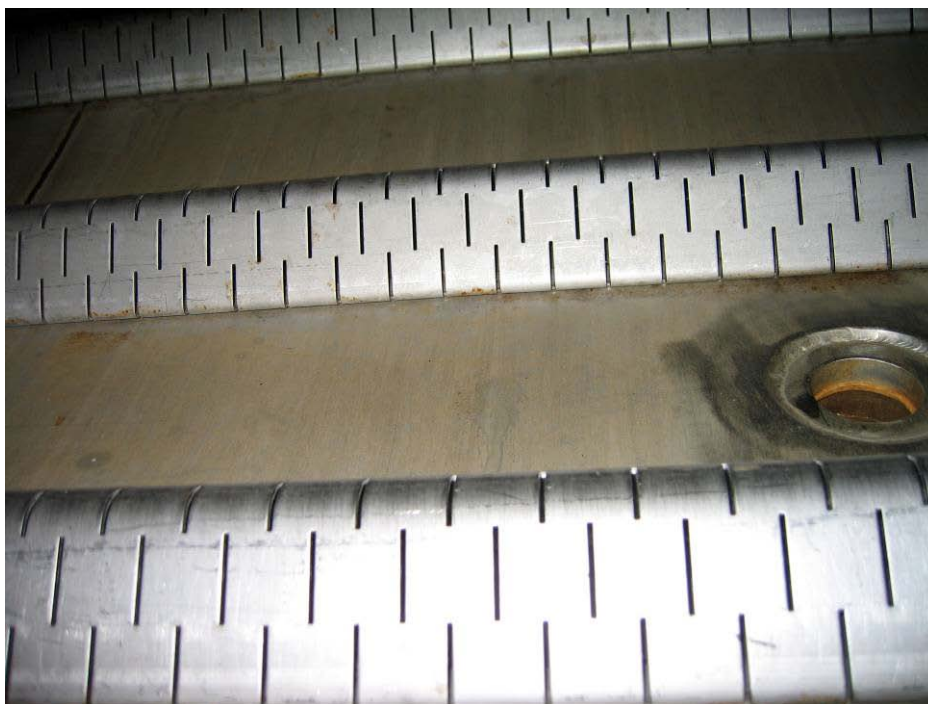
Figure 5.16: Drainage channels in a Bucher-Vaslin XP320 membrane press
