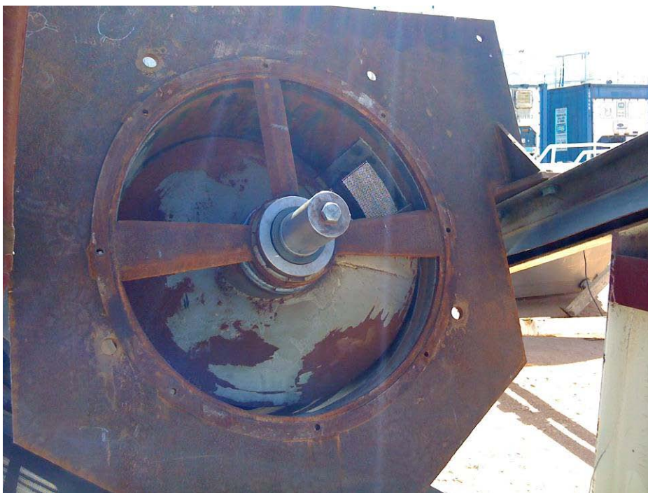
Figure 4.12: Static anti-return device on a partially disassembled inclined drainer
