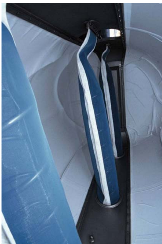
Figure 5.19: Vertical central flexi-drain juice channels in a Willmes press (From: Scott Laboratories 2010)
