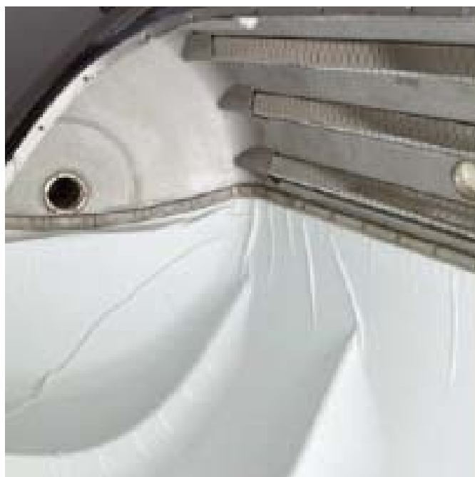
Figure 5.24: Spiral elements set under retracted press membrane to convey pressed pomace to exit door(s) during emptying by tank rotation (From: Bucher-Vaslin 2010b)
