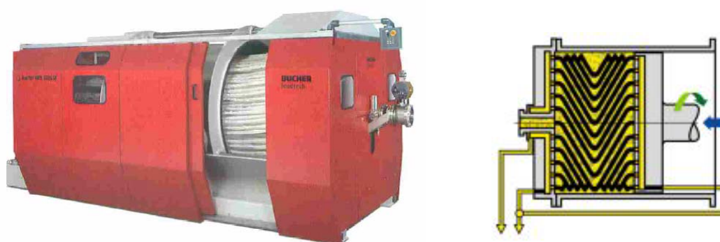
Figure 8.1: Bucher HPX 5005iP horizontal hydraulic single plate press with cloth covered drainage cores and schematic of operating principle
