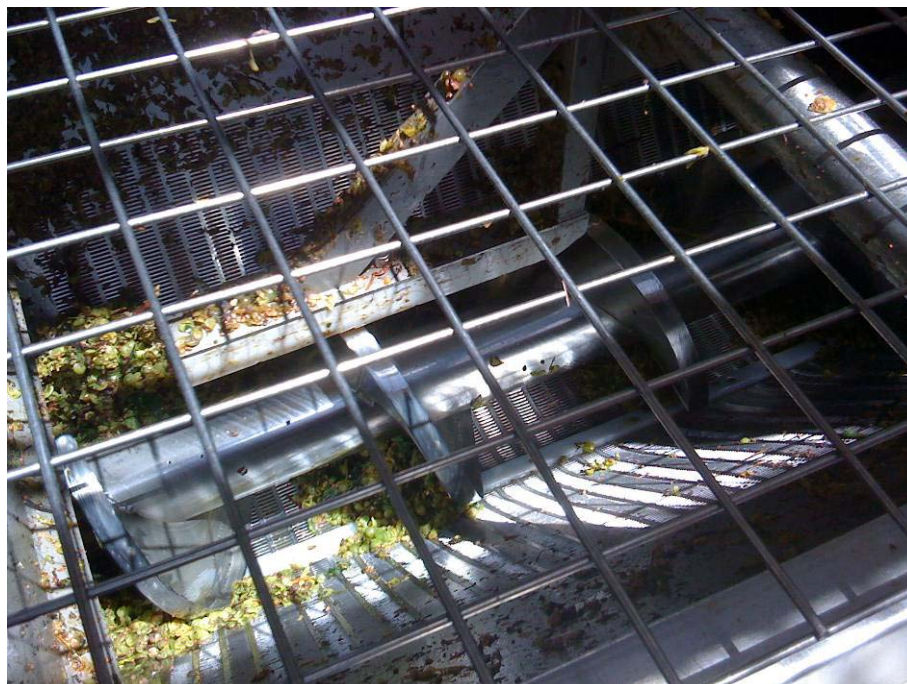
Figure 7.4: Draining section at feed to destemmer-crusher
