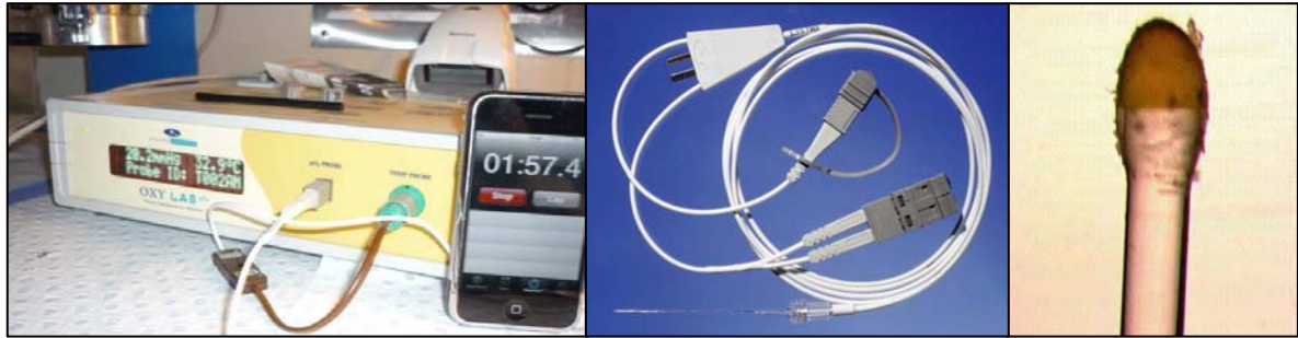
Figure 5.4. The OxyLab system fibre optic probe manufactured Oxford Optronix Ltd (230 \mu\text{m} width shaft and 280 \mu\text{m} tip diameter) used for in vivo \text{pO}_2 measurement.
