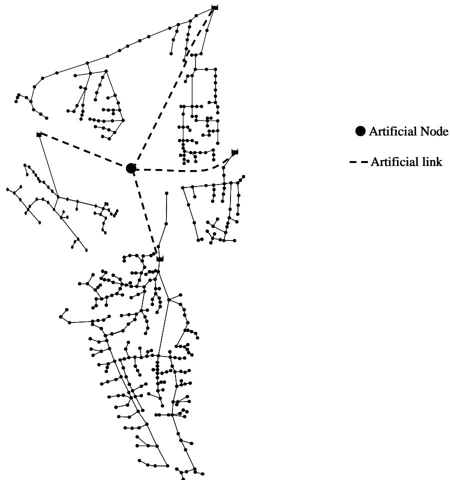
Figure 10 The layout of the shortest-distance tree of the Balerna network
