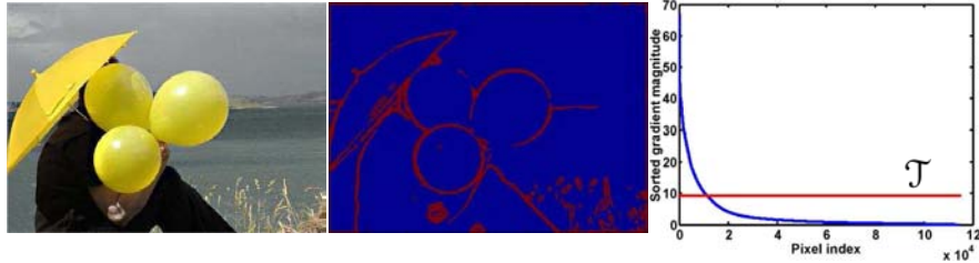
Figure 3.4: Illustration of the gradient magnitude information for hyperedge saliency evaluation. The left subfigure shows the original image, and the middle subfigure displays the gradient magnitude map I_g^* obtained by binarizing I_g using the adaptive threshold \mathcal{T} , as illustrated in the right subfigure.
