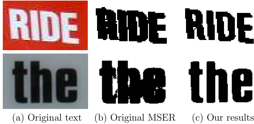
Figure 4.2: Cases that the original MSER fails to extract the characters while the modified eMSER succeeds.
