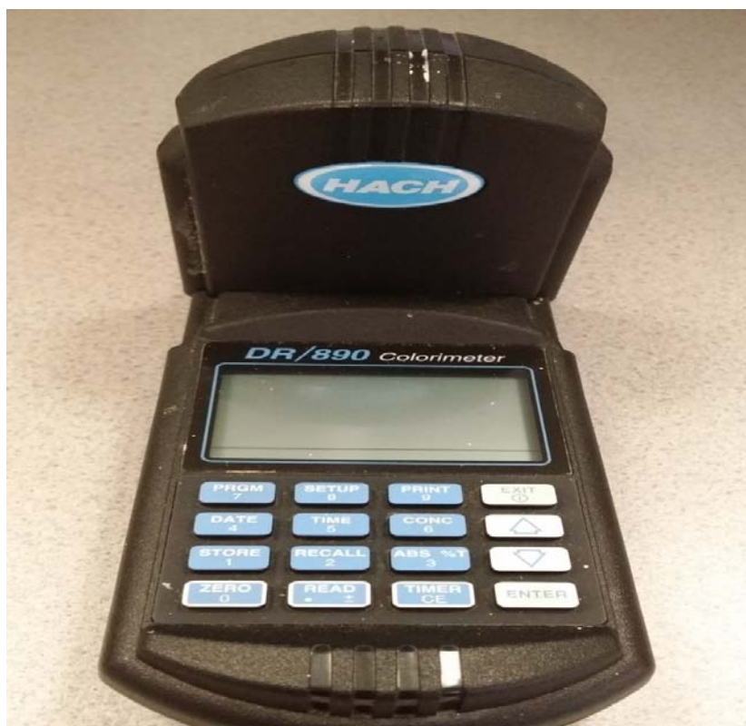
Figure 3.4 Colorimeter HACH used to measure \text{NH}_4^+
