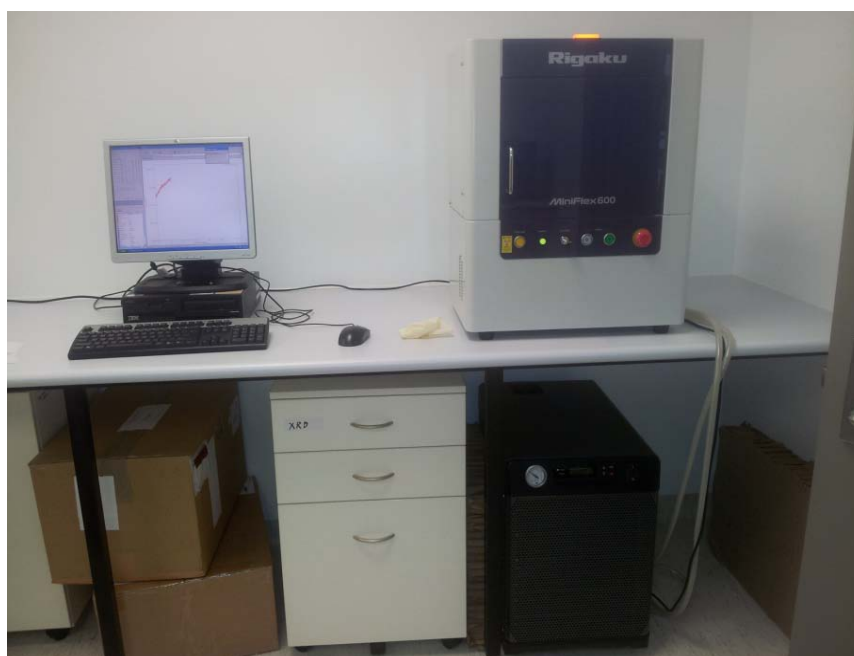
Figure 3.5 X-ray Diffraction, Miniflex 600 used to identify struvite, magnesite and struvite-(K).
