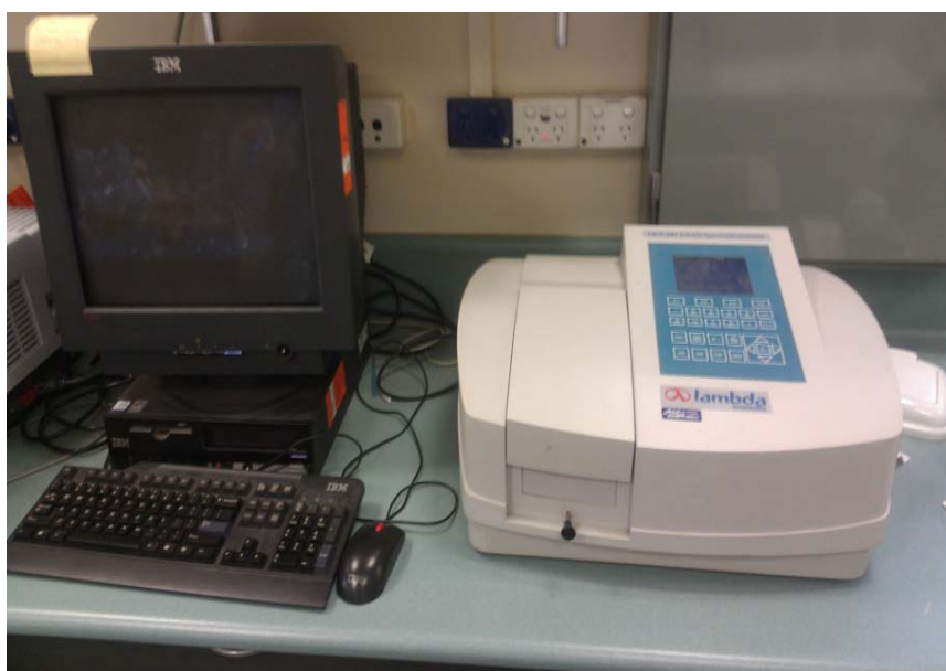
Figure 3.3 LIUV-201 UV/Vis spectrometer used to measure PO_4^{3-}
