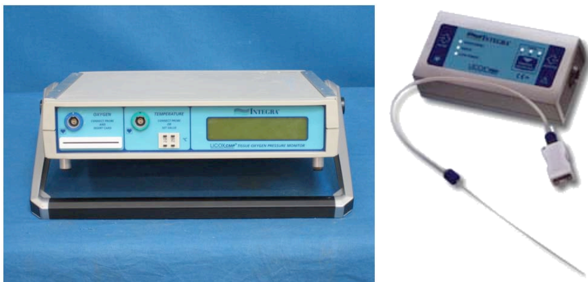
Figure 1.3: The Integra™ Licox® system. The oxygen-sensing probe (model CC1.P1) sits at the tip of the slender microcatheter (right), which is implanted within the brain parenchyma. The distal end of the probe is connected via cable to the CMP monitoring unit (left) for continuous real-time measurement of brain tissue oxygen concentration.
