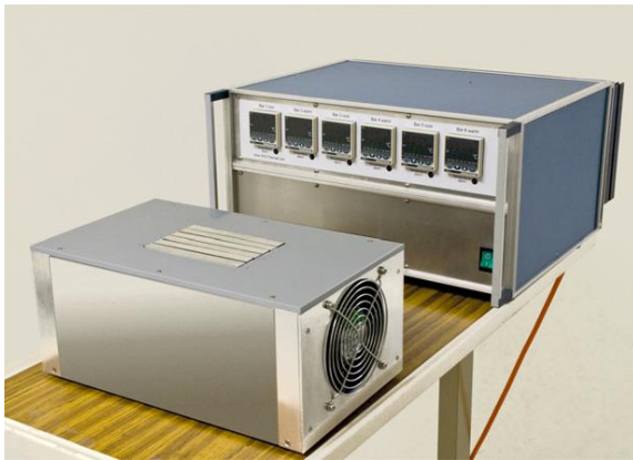
Figure 1 Image of the thermal grill. In the center of the Bar Box (smaller box) is the stimulation surface, where participants were required to place their nondominant palm orthogonally to the long axis of the bars. The stimulation surface consists of six 12-mm wide and 120-mm long aluminum bars separated by approximately 2 mm of thermal insulation. The Control Unit (larger box) set the temperature of the individual bars to alternating cool and warm temperatures.
