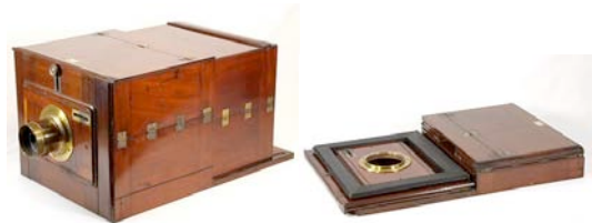
Plate 8b Thomas Ottewill & Co. Folding Sliding Box Camera for collodion wet plates, 1853
