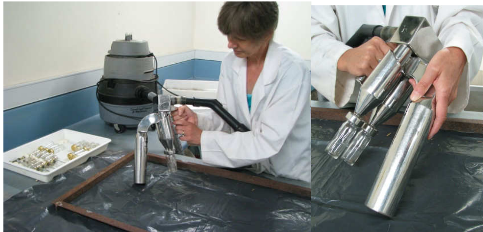
Figure 6-3 Suction device used to remove dust, collected onto plastic sheets placed in a transect from the edge of a field pea crop in Kingsford during harvest, into glass vials
