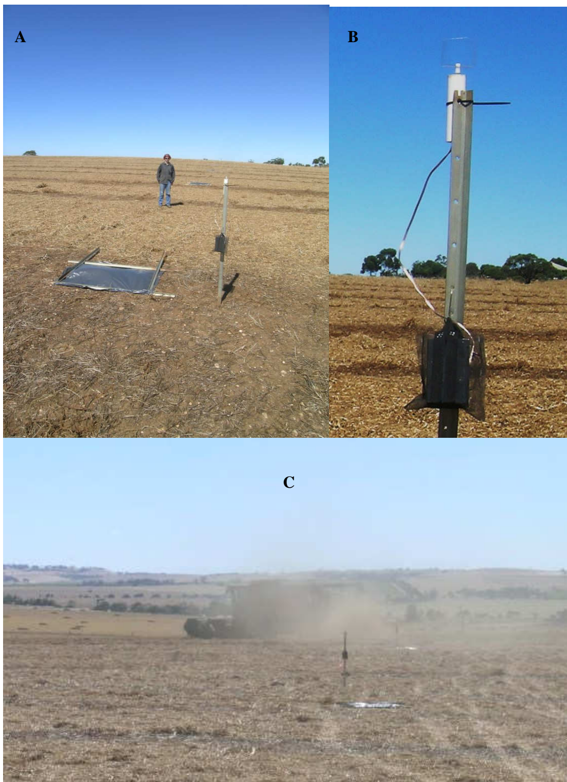
Figure 6-4 Sampling of dust generated during harvest of a field pea crop at Kingsford, December 2009. A. Transect of plastic sheets and rotorod samplers at right angles from the edge the field B. Rotorod sampler with battery mounted on post C. Transect of plastic sheets and rotorod samplers with harvester generating dust visible in the crop behind
