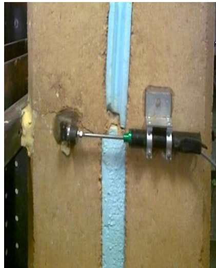
35 Figure 13 LVDT for recording the relative displacement of two RE wall leaves 36
