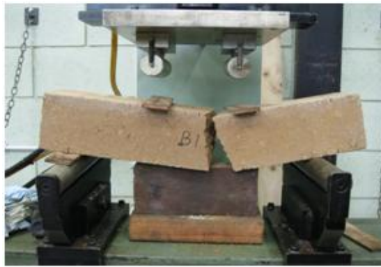
(b) Failure pattern of beam specimens
