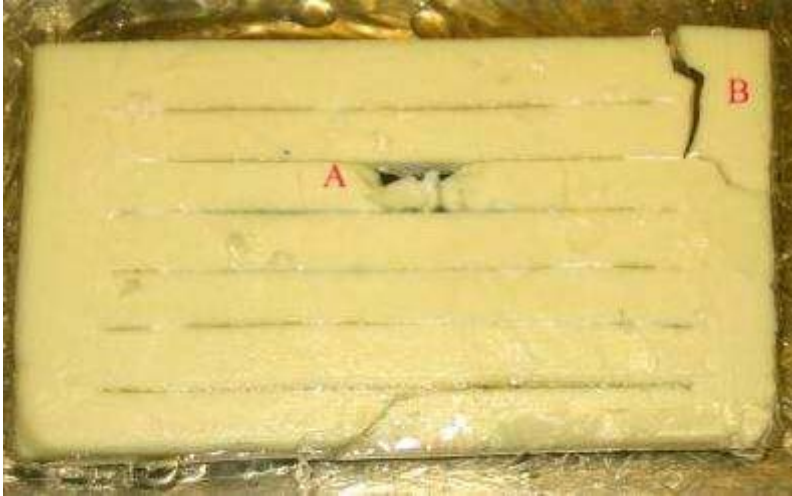
Figure 41. Test 7. Point A indicates the exit point of the ASF1 ball bullet through the bone composite which was embedded within the anterior gelatine plate. Point B indicates the remote damage caused to the bone composite through the transfer of energy from the shock wave associated with temporary cavitation.
