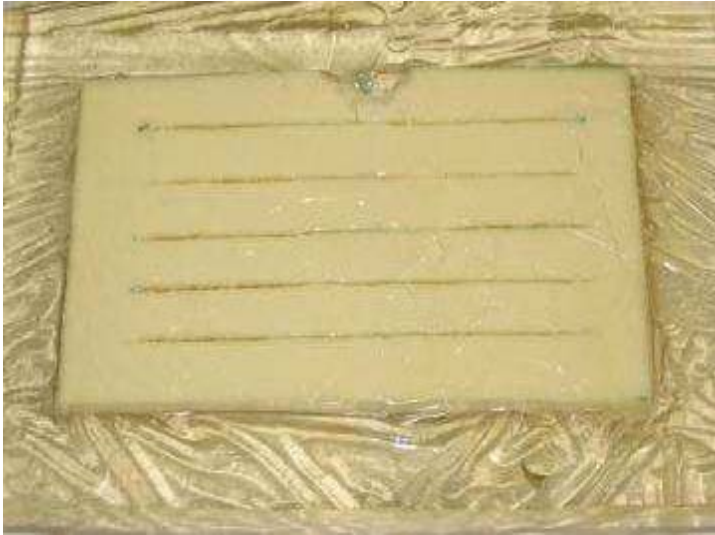
Figure 7. A sample of the bone composite embedded within a thin gelatine plate.
