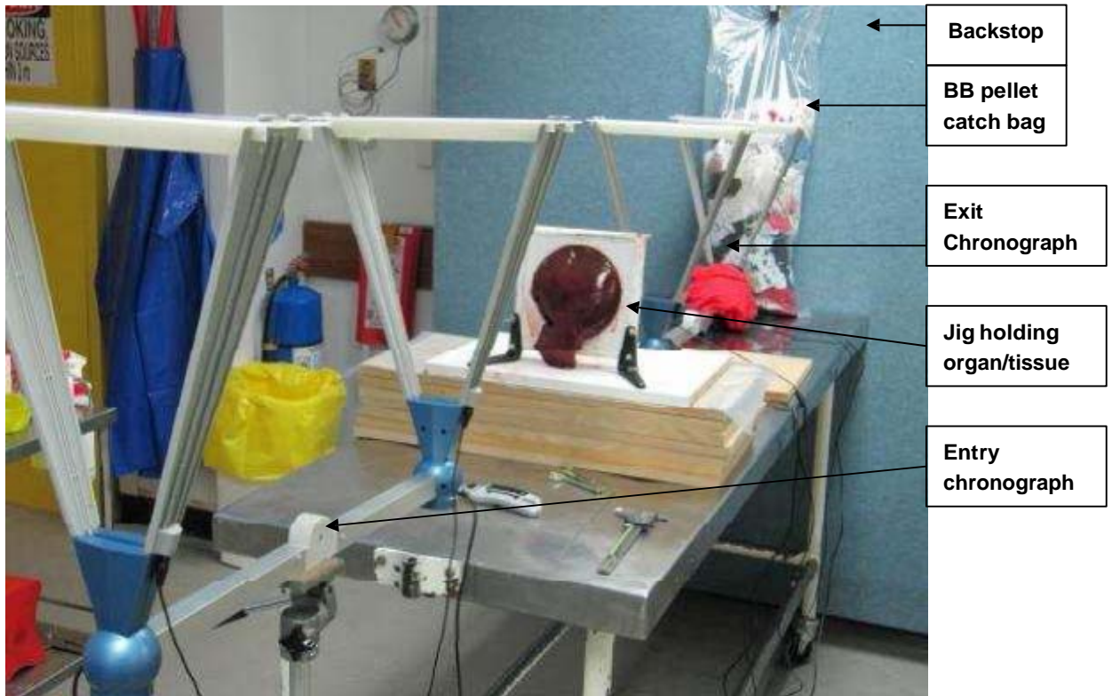
Figure 4. Closer view of velocity testing equipment (chronographs) and tissue/organ/simulant apparatus.
