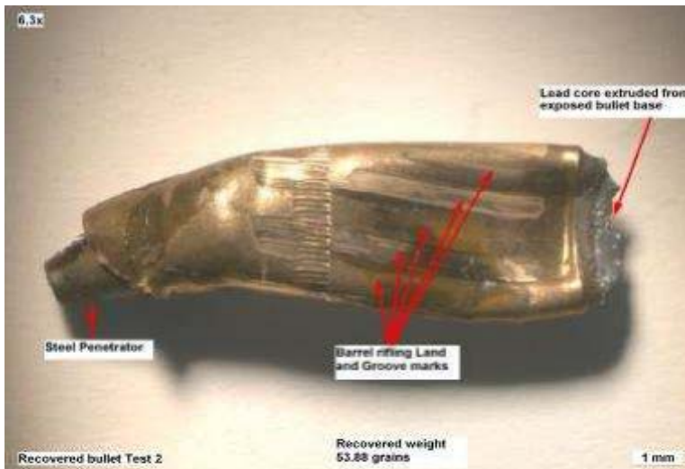
Figure 46. Test 2. Recovered ASF1 ball bullet. The bullet is deformed and the jacket around the forebody has torn to reveal the steel penetrator. Lead from the internal base core has been extruded from the base of the bullet and was found within the permanent cavity. Total retained bullet weight = 87% of the original weight.
