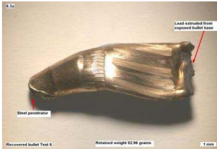
Figure 47. Test 6. Recovered ASF1 ball bullet. The bullet is deformed and the jacket material around the forebody has torn to reveal the steel penetrator. Lead from the internal base core has been extruded from the base of the bullet and was found within the permanent cavity. Total retained bullet weight = 85% of the original weight.
