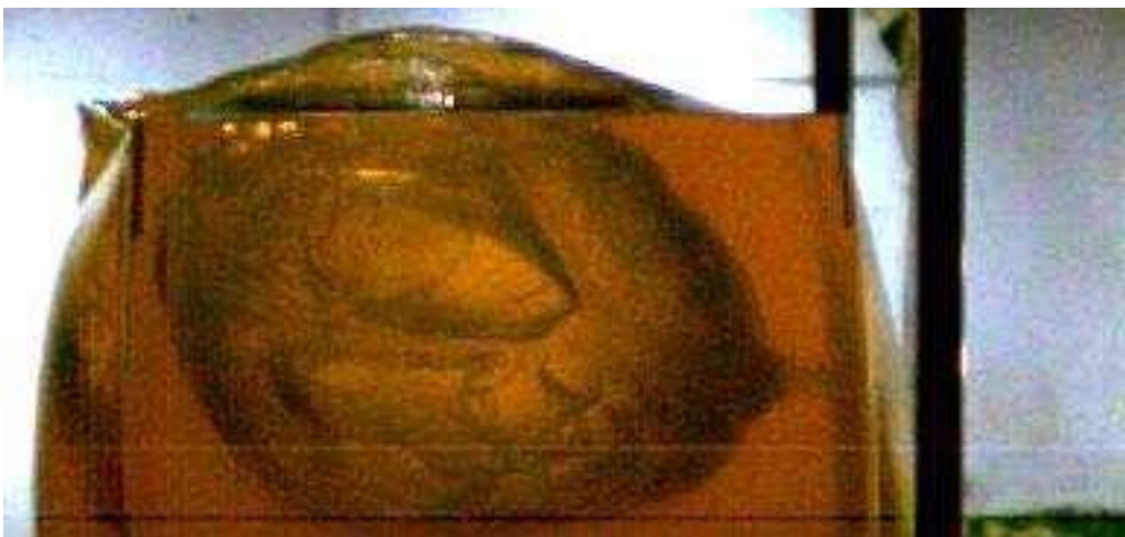
Figure 26. Test 1A. Point at which maximum temporary cavitation has occurred within the bare gelatine block.
