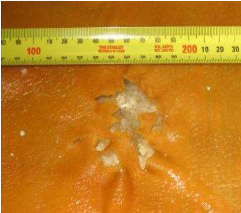
Figure 43. Test 7. The extensive damage caused by the ASF1 ball bullet at maximum yaw as it exited the skin simulant attached to the back of the posterior gelatine plate.
