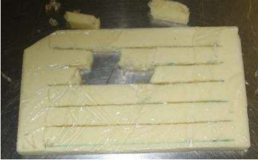
Figure 33. Test 5. Bone composite that was embedded within the gelatine plate showing a large area of damage.
