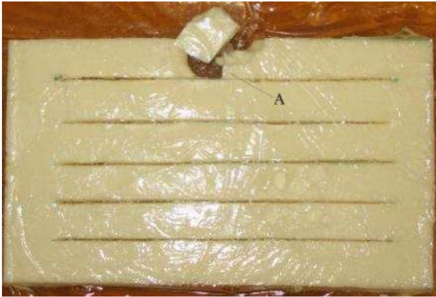
Figure 36. Test 6. Point A indicates the damage sustained to the bone composite embedded within the gelatine plate.
