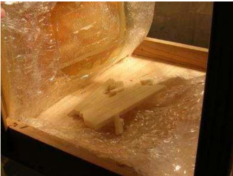
Figure 42. Test 7. The extensive damage caused by the ASF1 ball bullet to the bone composite embedded within the posterior gelatine plate.
