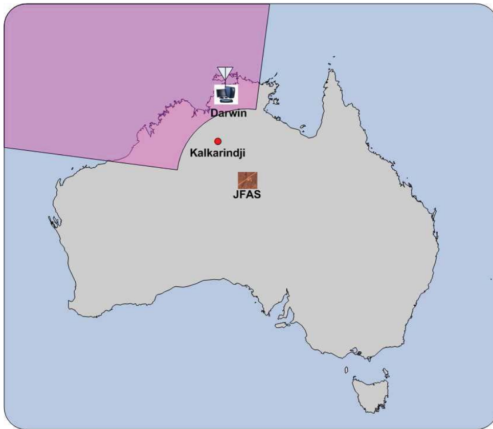
Figure 5.2. The location of the JFAS radar transmitter and the CCP in Darwin. Transmitter coverage is shown in magenta. Kalkarindji is the location of the ionosonde from which the ionospheric parameters of the path were recorded.
